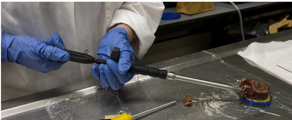
Figure 36 | TIVAD Inserter (Concept 3) & Expander (Concept 1, still with straight handle) in action
