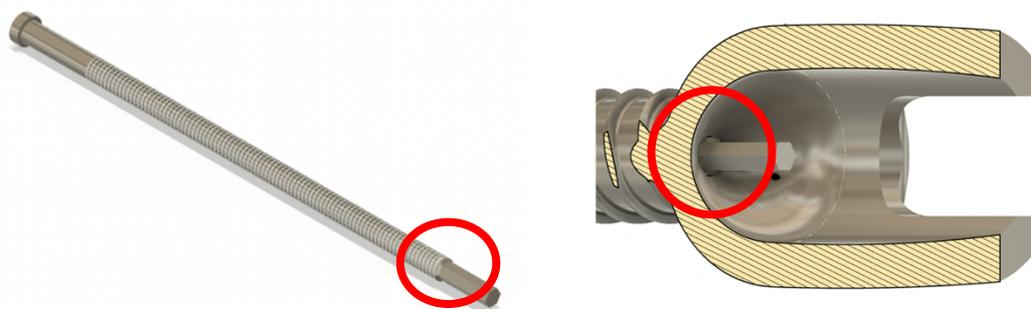
Figure 37 | TIVAD expansion screw (left), inside TIVAD implant (right)
