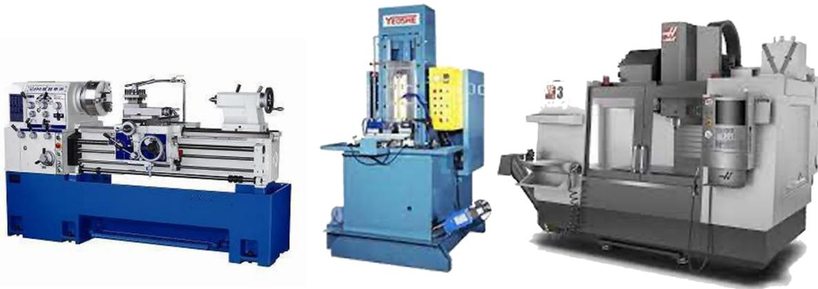
Figure 40 | Turning machine (left), Broaching machine (middle), 3-axis CNC (right)
