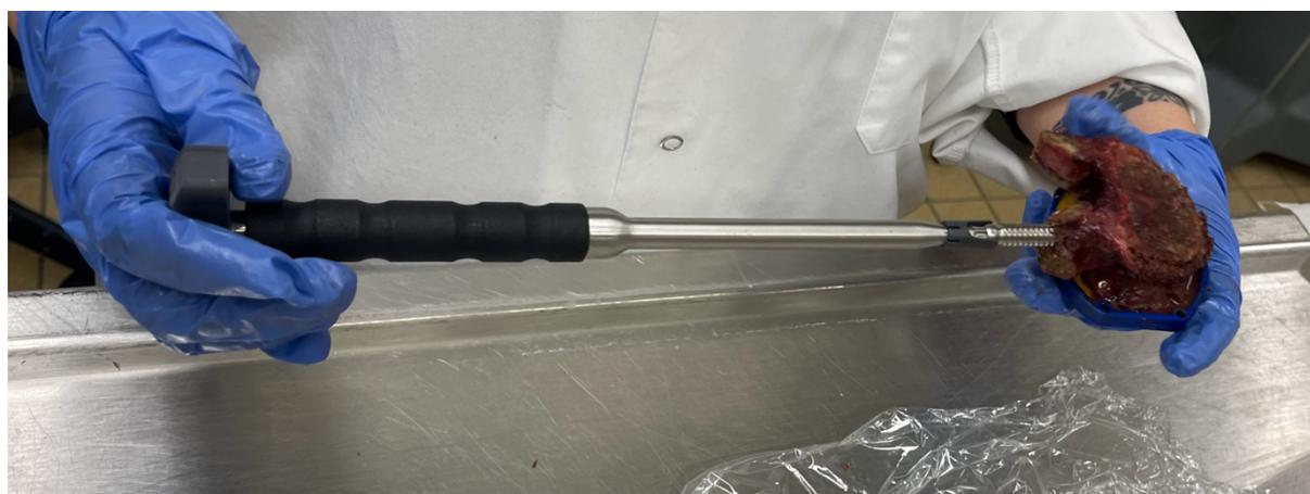
Figure 46 | Experimental test with TIVAD Inserter and CVB in a horizontal position
