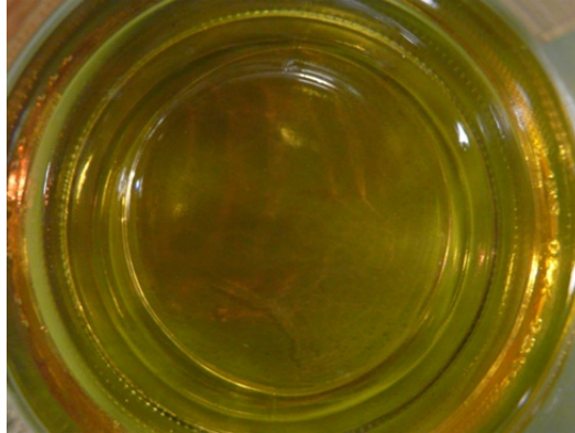
Figure 4-3. Sludge in mineral oil
