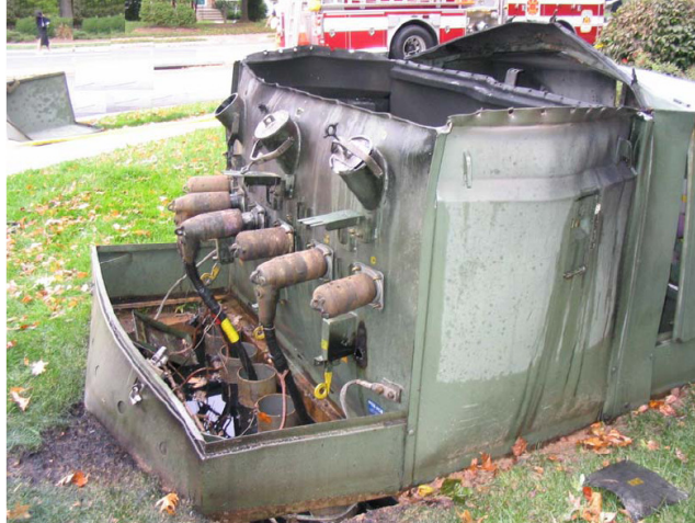
Figure 1-9. Mineral oil leakage after a 19 kV transformer explosion
