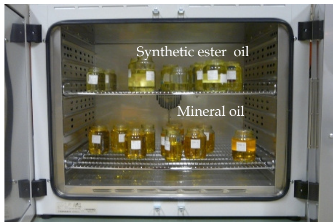
Figure 3-2. Photo of oil samples in the oven for accelerated aging process
