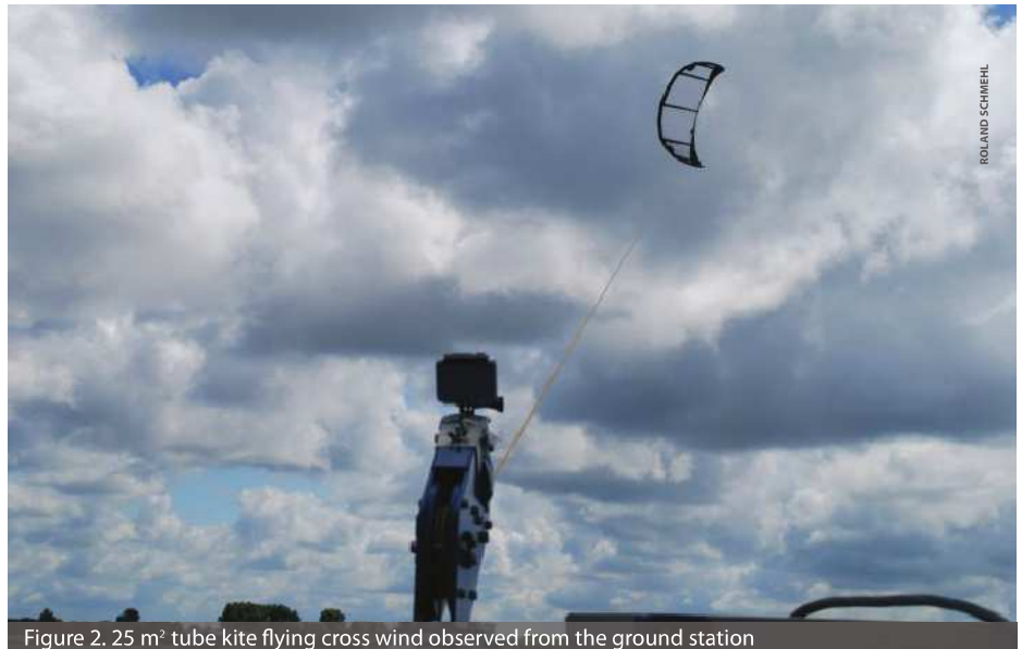
Figure 2. 25 m 2 tube kite flying cross wind observed from the ground station
