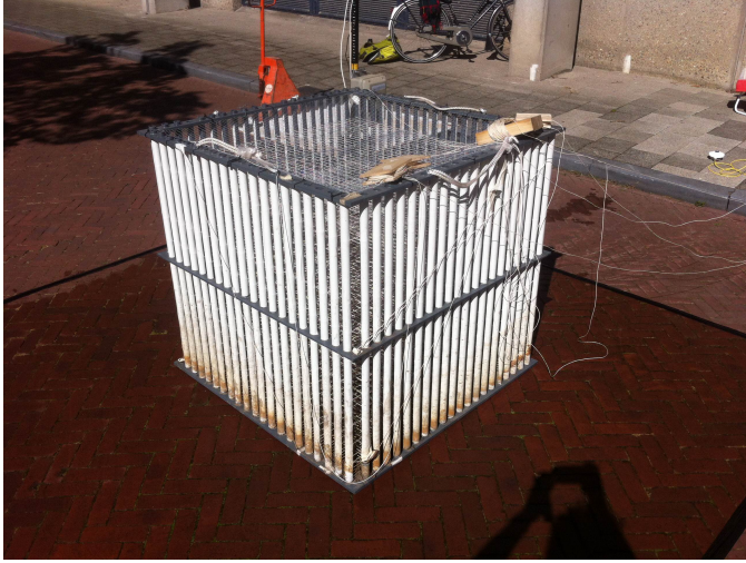
Figure 5.2: Measurement setup, consisting of the cage construction ( 1\text{m}^3 ) during the experiments.
