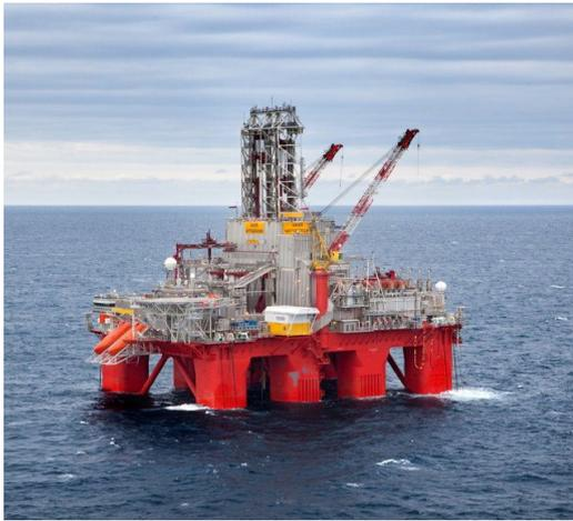
Figure 1.1: The “Transocean Spitsbergen”, a semi-submersible drilling rig capable of drilling at a water depth of 3 kilometres. (Image from Equinor / Kenneth Engelsvold)
