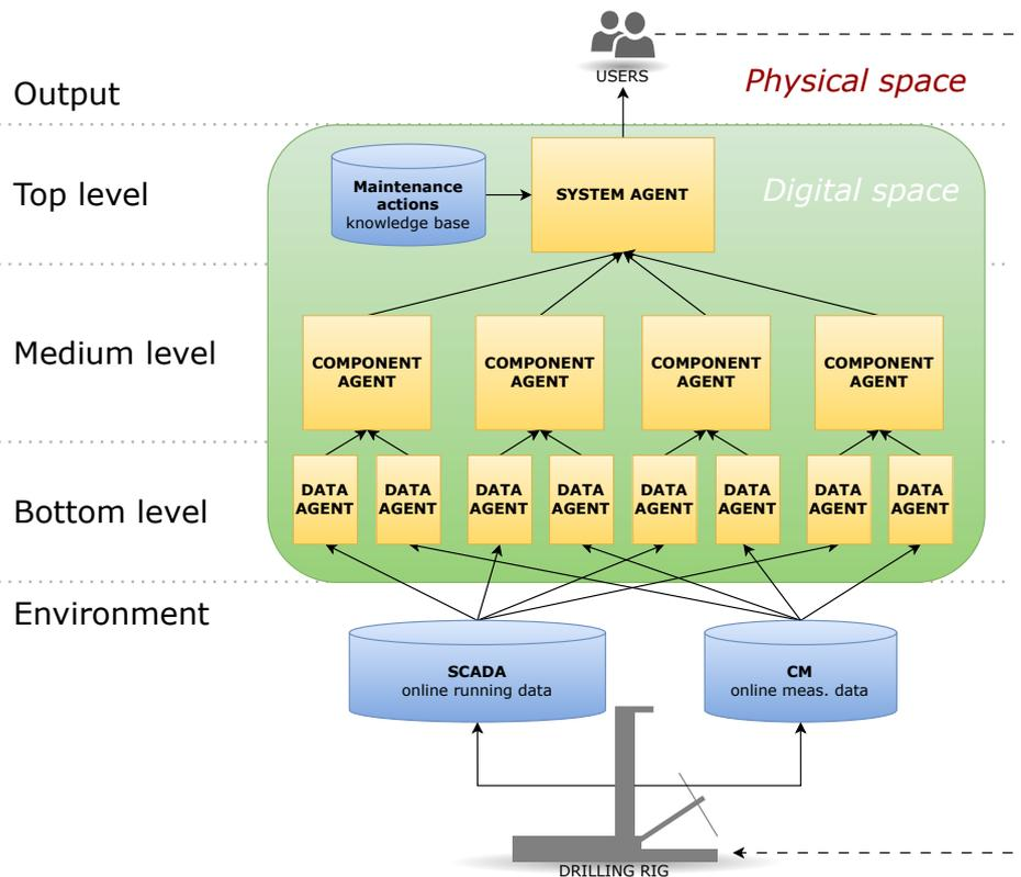
Figure 4.4: The hierarchical multi-agent system framework proposed in this thesis.
