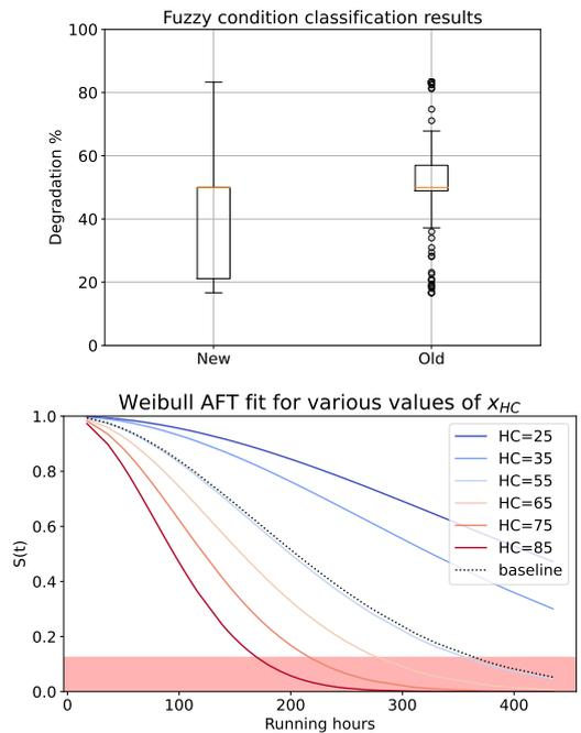
Fig. 12. WAFT survival functions, RUL threshold indicated in red.
