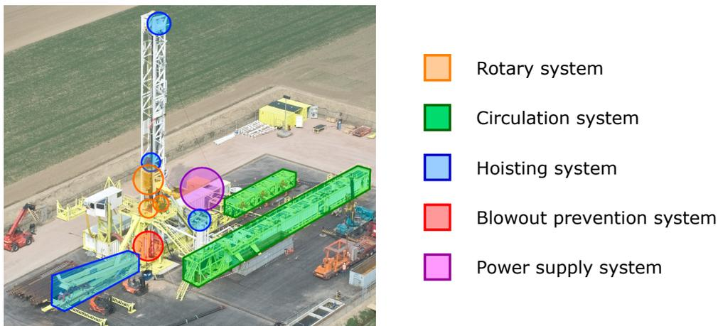
Figure 2.1: The five subsystems on a drilling rig system, the typical locations on the rig are highlighted (Image from Huisman Equipment)
