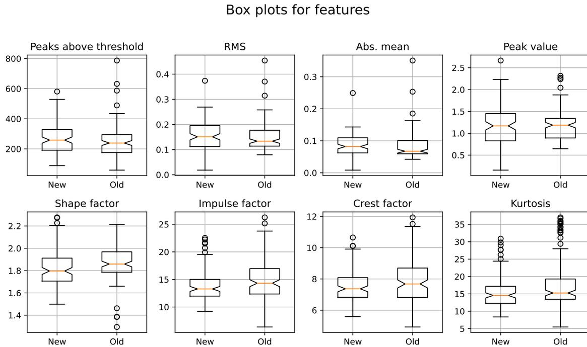
Figure 6.7: Various features extracted and box plotted from vibration signals of old and new mud pump valves.
