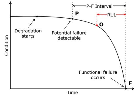
Fig. 3. A general P-F curve: relation between observance of a potential failure (P) and the actual failure (F). The RUL from a certain observation (O) is highlighted as well. (Image based on [15])
