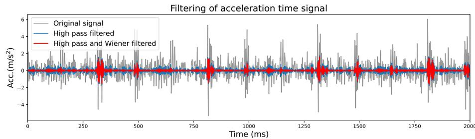
Figure 6.6: One second sample of a time series signal, first filtered by a high-pass filter and subsequently by a Wiener filter.
