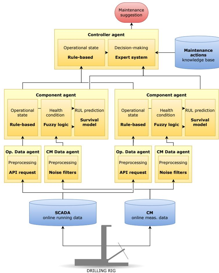
Figure 5.6: Overview of the proposed model, including the demanded functions per agent. The methods to perform these functions are given as well. Information flow is indicated with arrows.
