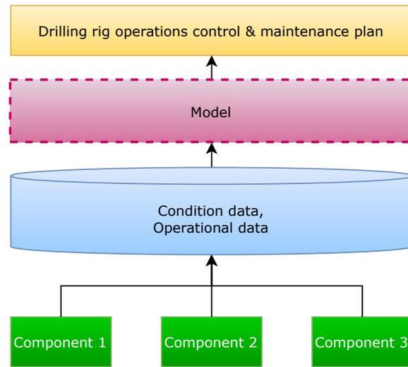
Figure 1.4: Desired situation: data is analysed in a single model, maintenance decisions are integrated in the system control
