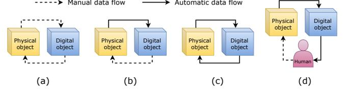
Fig. 5. Classification of DT based on level of data integration: (a) Digital model, (b) Digital shadow, (c) DT and (d) DT with human integrated in the decision loop. (Image based on [36]–[39])
