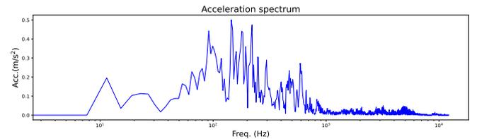
Fig. 8. Example of acceleration FFT spectrum acquired from mud pump vibrations
