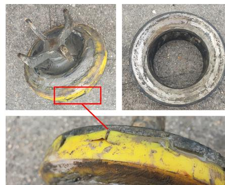
Figure 6.2: Worn mud pump valve and seat. On the seat (top-right), starting corrosion is visible. The plastic valve insert is torn. (Image taken during field research)
