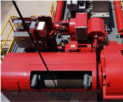
Figure 2.3: This drawworks is driven by two motors and has a rating of 1800 horsepower. (Image from NOV)
