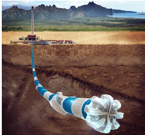
Figure 2.8: The Bottomhole Assembly of a Rotary Steerable System. (Image from NOV)
