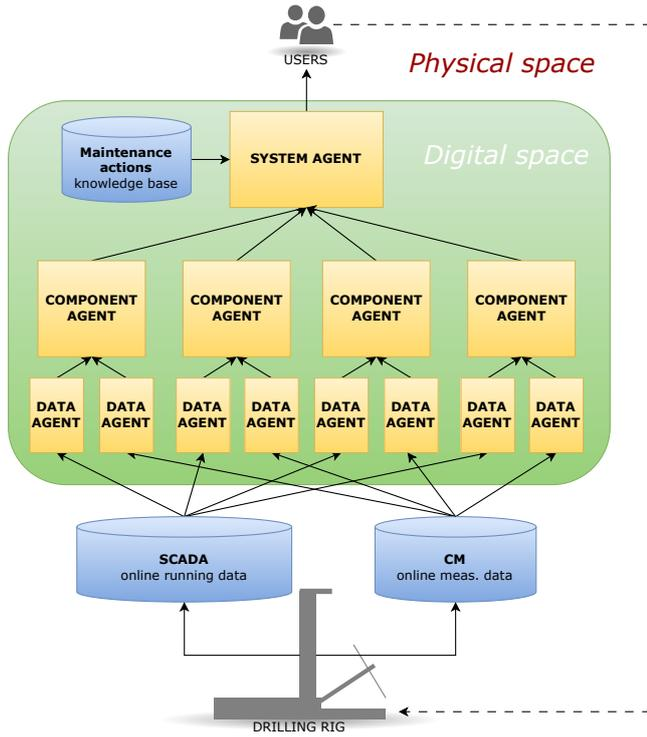
Fig. 6. The centralised MAS-DT framework proposed in this work.
