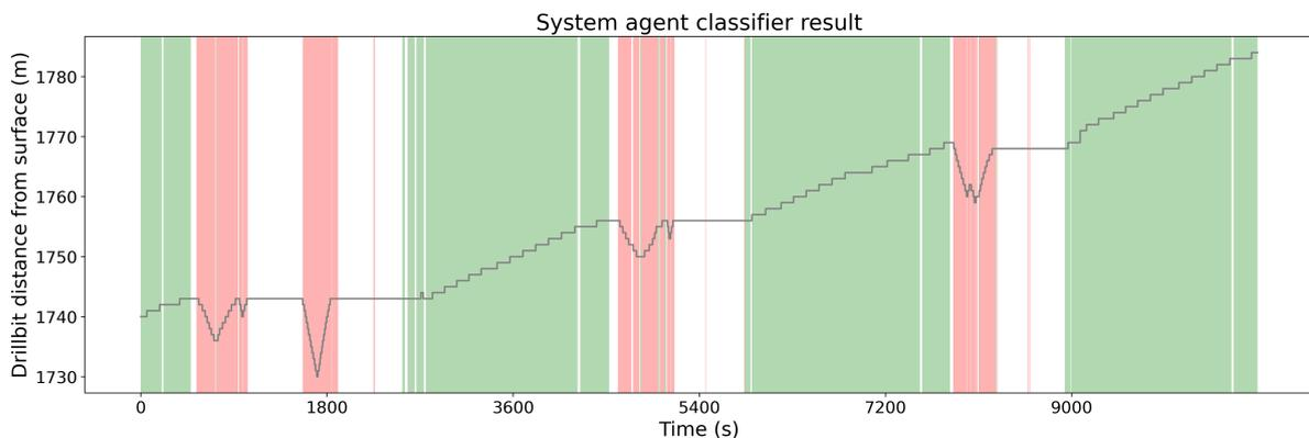
Figure 6.12: The result of the system operational state classifier. Green indicates drilling, red indicates tripping. The input for this classification are the parameter values in Figure 6.4. The drillbit location is plotted as well to validate the classification.
