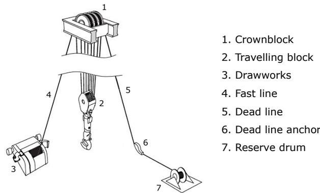
Figure 2.2: Schematic overview of components in a hoisting system
