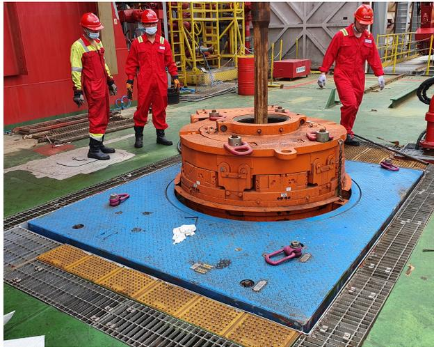
Figure 2.6: Offshore rotary table with power slips.
