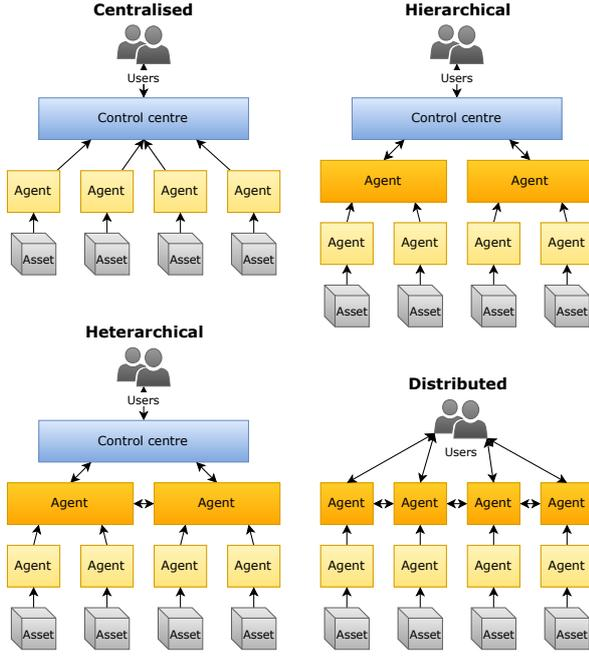
Fig. 4. Four types of MAS in PdM (Image based on [33])
