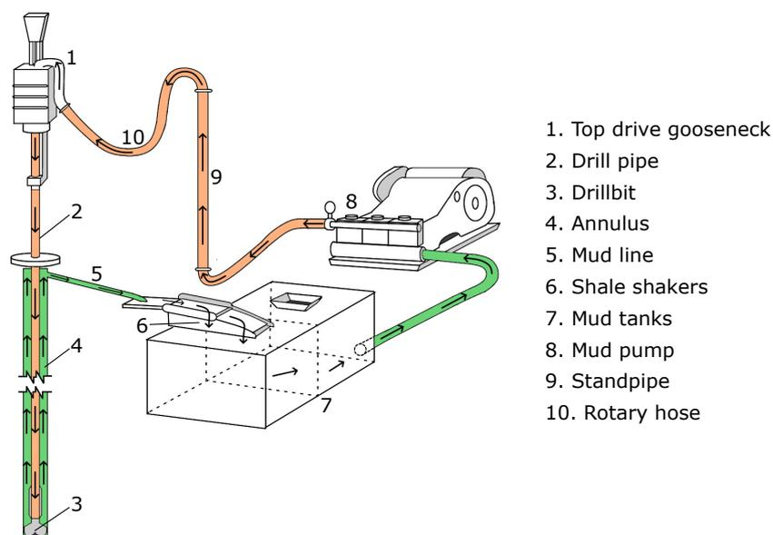
Figure 2.9: Schematic overview of a typical circulation system in a drilling rig. The mud flow is indicated with arrows and colours to indicate the state of the mud. (Image based on [35])
