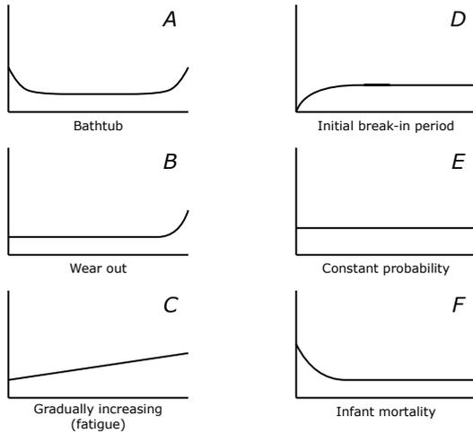
Fig. 2. Pattern curves of failure probability over time. Patterns A,B and C show a probability of failure related to equipment age. The failure probability patterns D, E and F are mostly constant, therefore they do not relate to age. (based on [11], [26])
