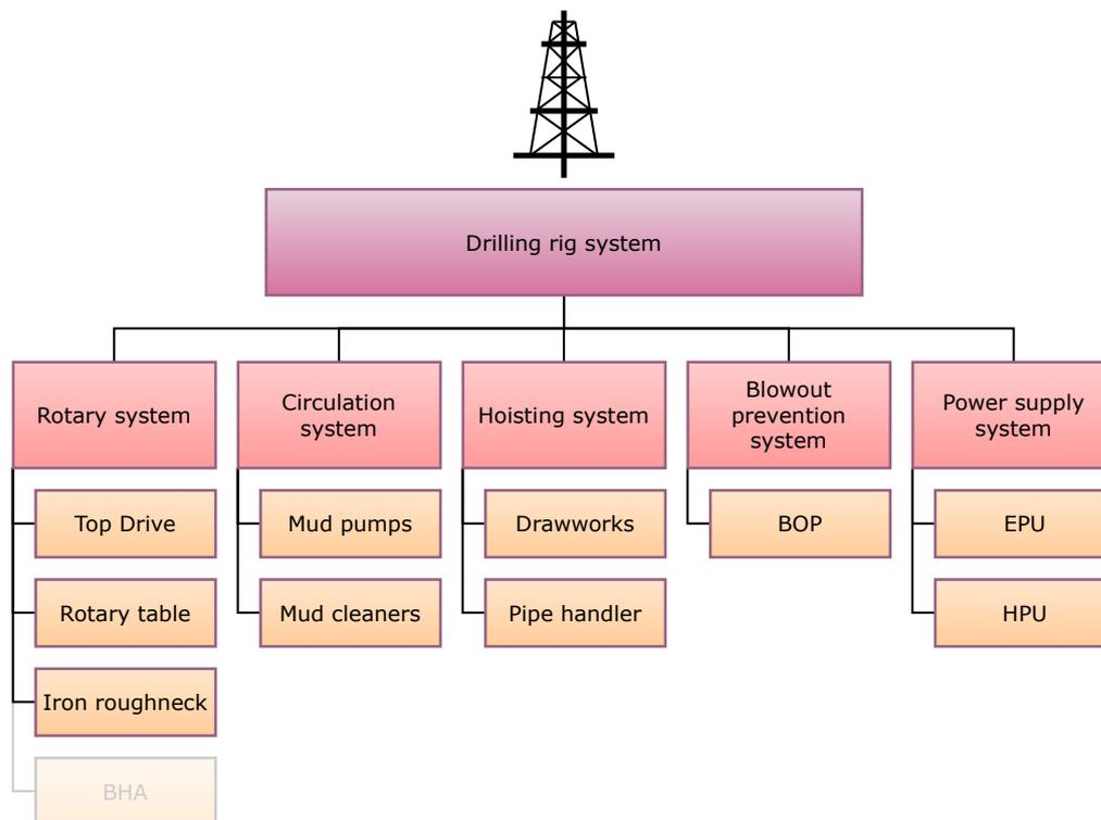
Figure 2.11: The critical components of a land drilling rig.
