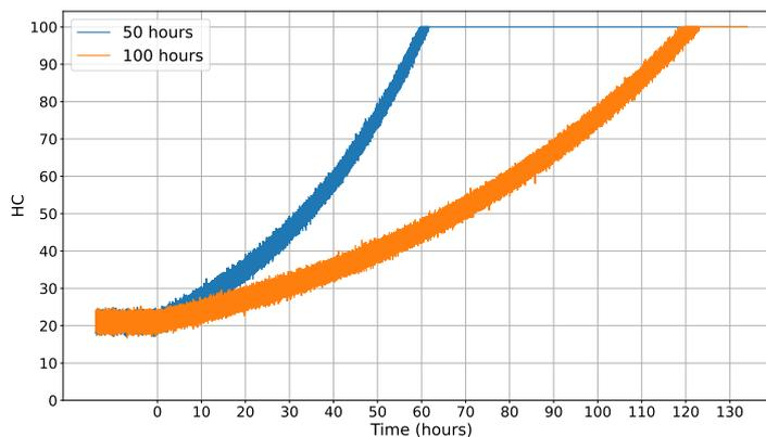
Figure 7.2: Plot of the artificially induced damage signal for the valves of a mud pump. At HC = 100 the valve has failed completely.
