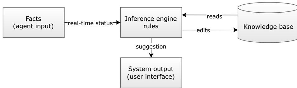
Figure 6.13: Schematic architecture of the reasoning system of the designed model.
