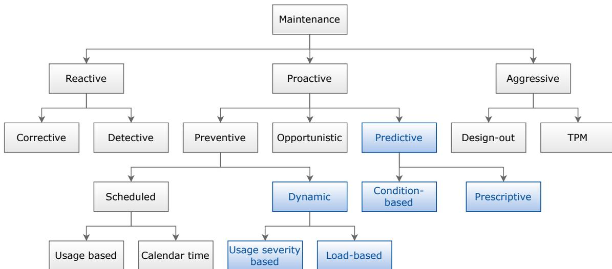
Figure 3.2: Overview and classification of different maintenance policies, based on Tinga [44, Chapter 5]. The advanced maintenance policies are highlighted in blue.
