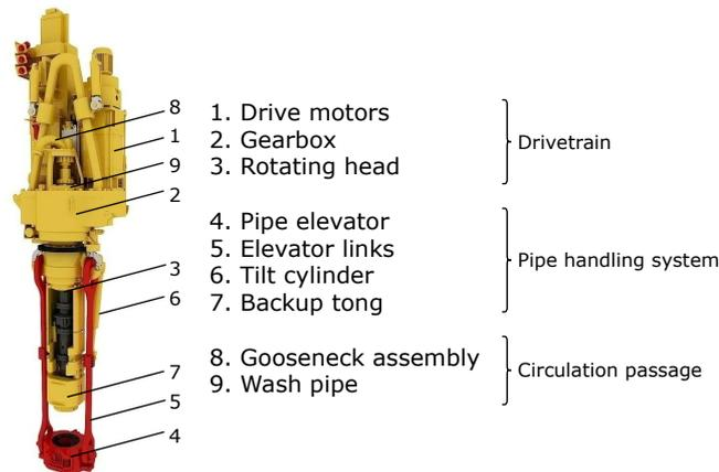
Figure 2.5: Overview of key components in a top drive system.
