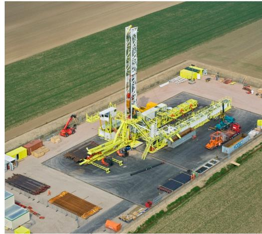
Figure 1.2: The Huisman LOC400 mobile land drilling rig. It has a relatively small footprint and features automated drilling systems. (Image from Huisman Equipment)
