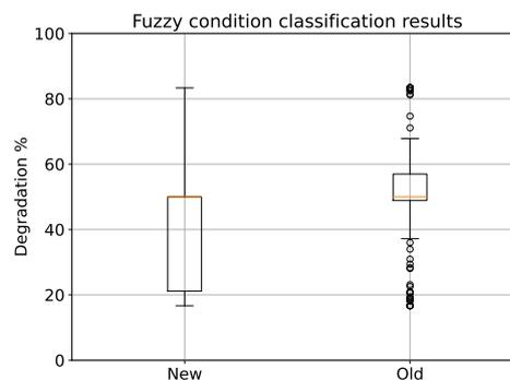
Figure 6.10: Results of the fuzzy classifier, box plotted for the old and new valve vibration samples.
