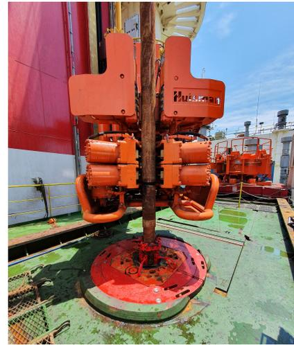
Figure 2.7: Offshore iron roughneck handling drill pipe. The drillstring is supported by manual slips.
