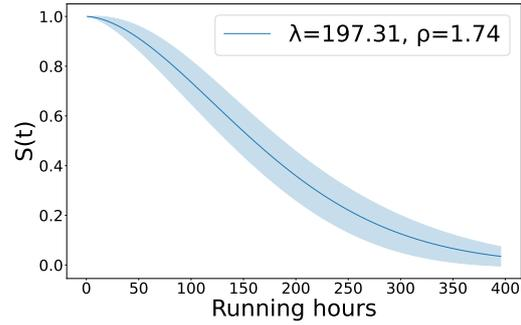
Figure 5.4: The Weibull survival function of the failure data presented in Figure 5.3.
