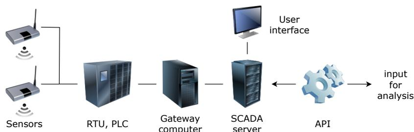
Figure 5.1: Schematic overview of the components in a SCADA system from sensor to API software.
