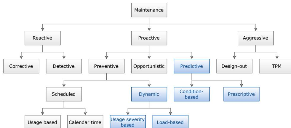
Fig. 1. Overview and classification of different maintenance policies, based on [15]–[17]. The advanced maintenance policies are highlighted in blue.
