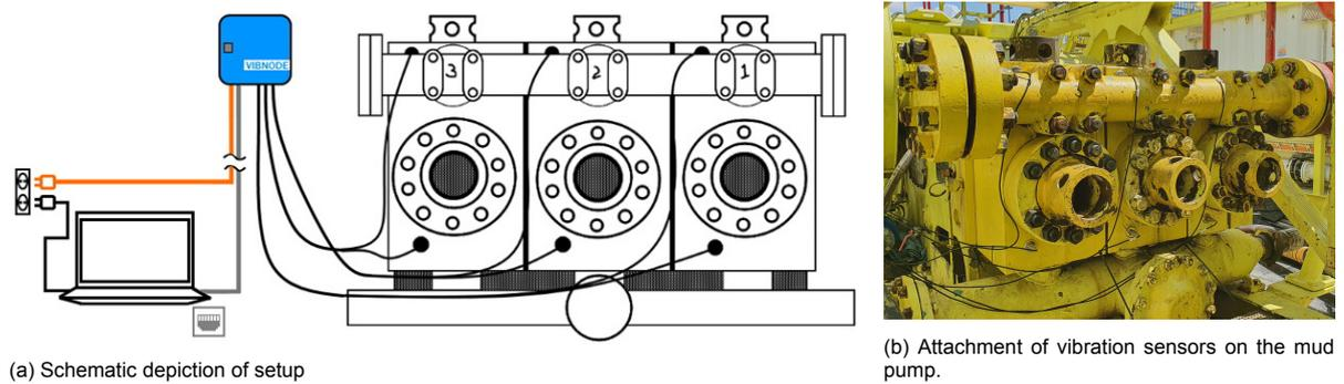
Figure 6.3: Overview of method for mud pump vibration data acquisition during the field research.
