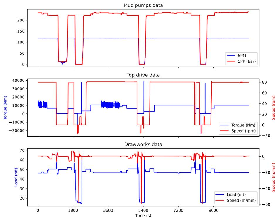
Figure 6.4: Parameters in operational data that are necessary for determining the rigs overall operational state, plotted per source component
