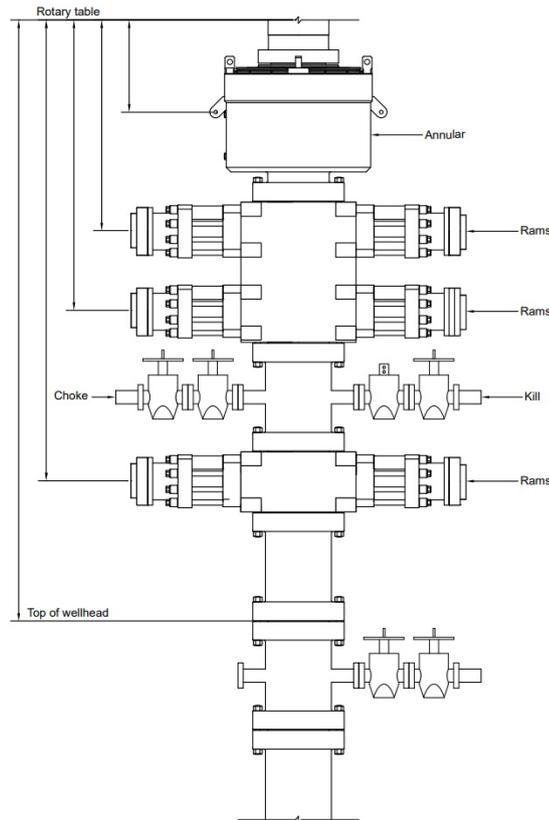
Figure 2.10: Typical surface BOP stack. (Illustration from API Standard 53, 2016, pp 45)
