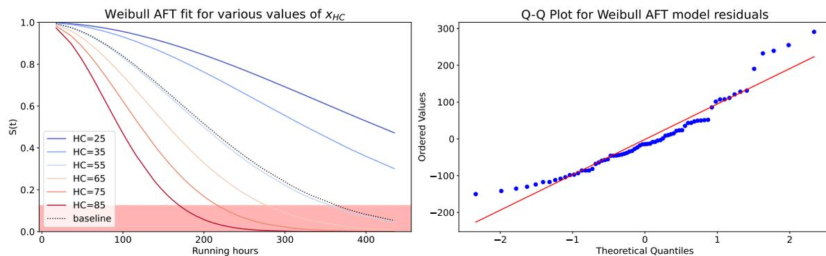
Figure 6.11: Result of the Weibull AFT fit. On the left, the partial effect of the health condition on the survival probability is plotted for various values of  $x_{HC}$ . The RUL threshold zone is marked in red. On the right is a Q-Q plot of the model residuals.
