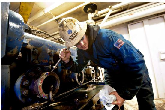
Figure 6.1: A driller is using a metal rod to listen to the fluid end of a mud pump. (Image from Bloomberg / Daniel Acker)
