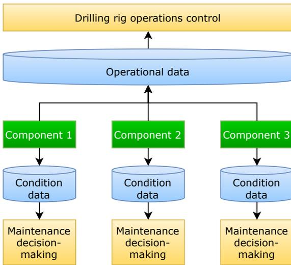
Figure 1.3: Current situation: maintenance strategies are on component level, system operations are not taken into account.
