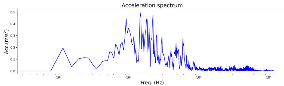
Figure 6.5: Acceleration spectrum of a mud pump. From this spectrum, it can be concluded that the lower frequencies of the acceleration signal are very dominant.
