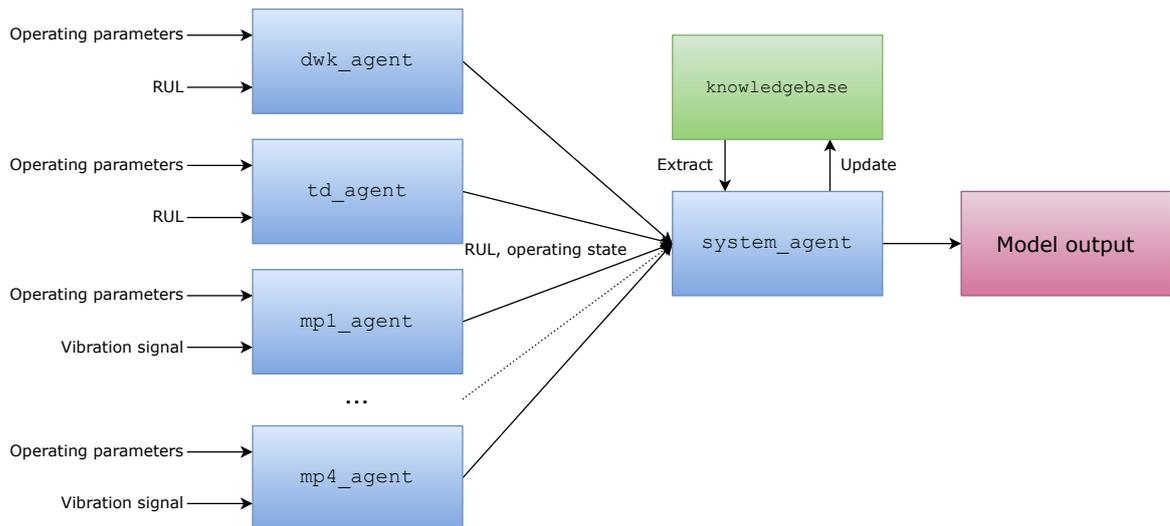
Figure 6.14: Structure of the realised software. Input parameters are depicted on the left and can be extracted from a dataset constructed from operational parameters extracted from SCADA and cleaned mud pump vibration signals.
