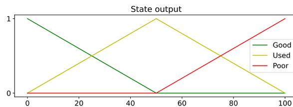
Figure 6.9: Fuzzy membership functions of the output state, corresponding to the estimated health condition of the valve.
