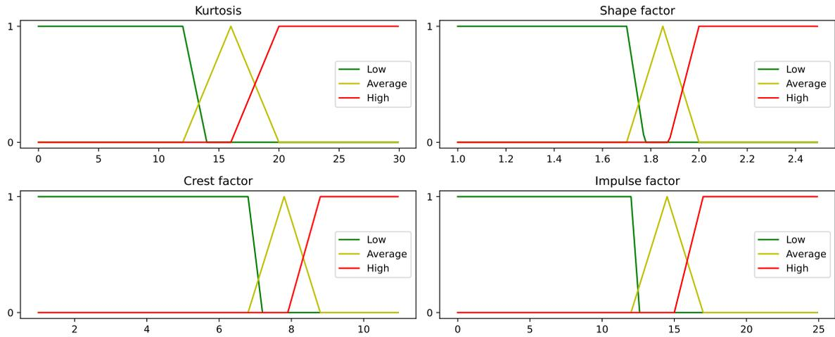
Figure 6.8: Fuzzy membership functions for the extracted feature kurtosis, shape factor, crest factor and impulse factor.
