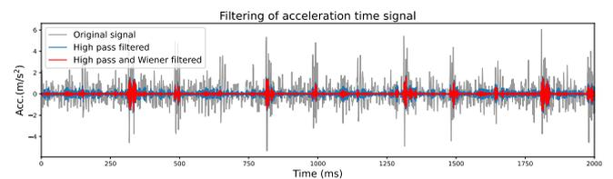
Fig. 9. Results after application of high-pass and Wiener filtering
