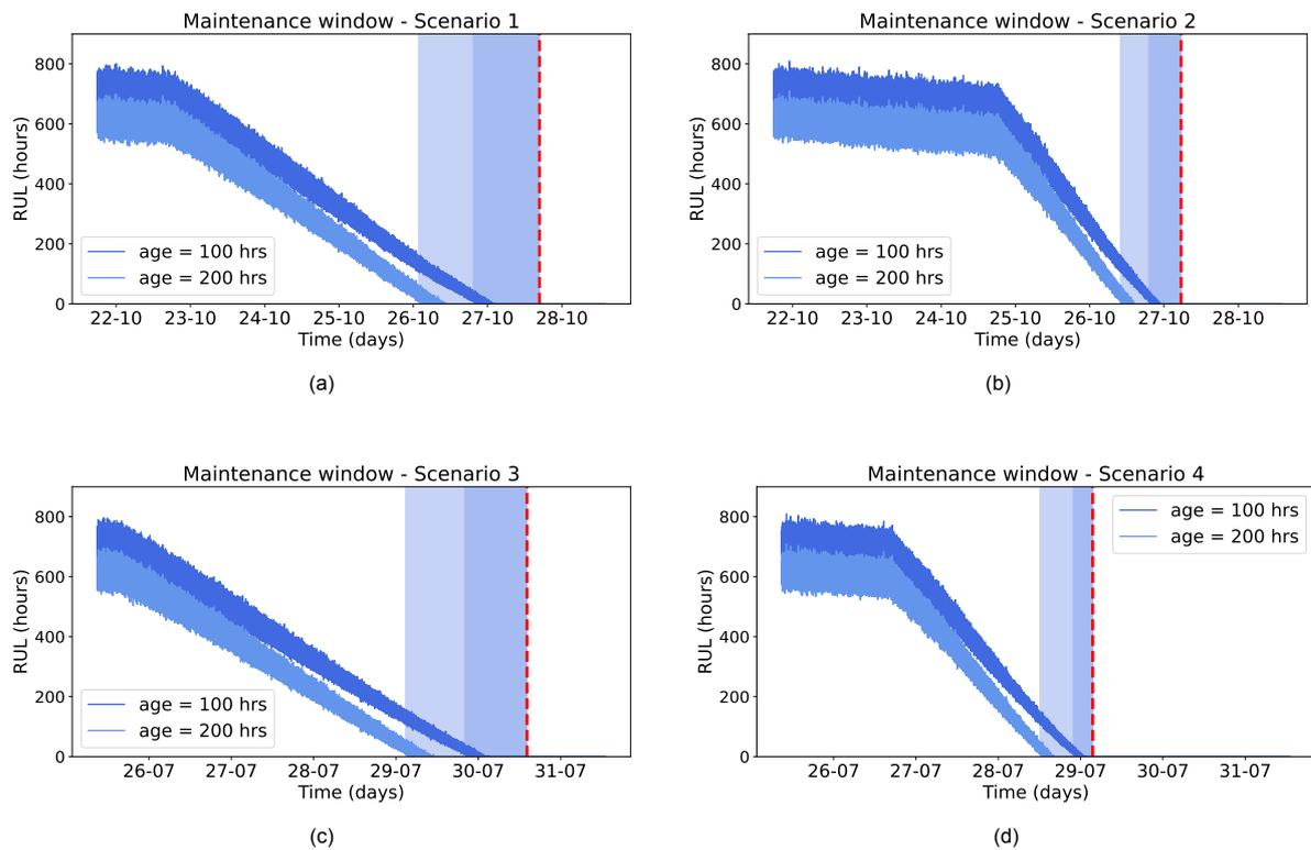
Figure 7.4: Maintenance windows suggested by the system agent when the RUL trigger for maintenance is 8 hours. Blue areas mark the maintenance window per component age. The red dashed line represents the theoretical moment of failure.
