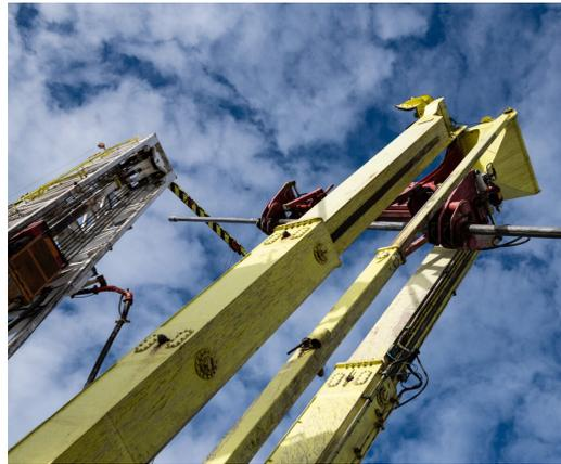
Figure 2.4: A horizontal to vertical pipe handling system. (Image from Huisman Equipment)
