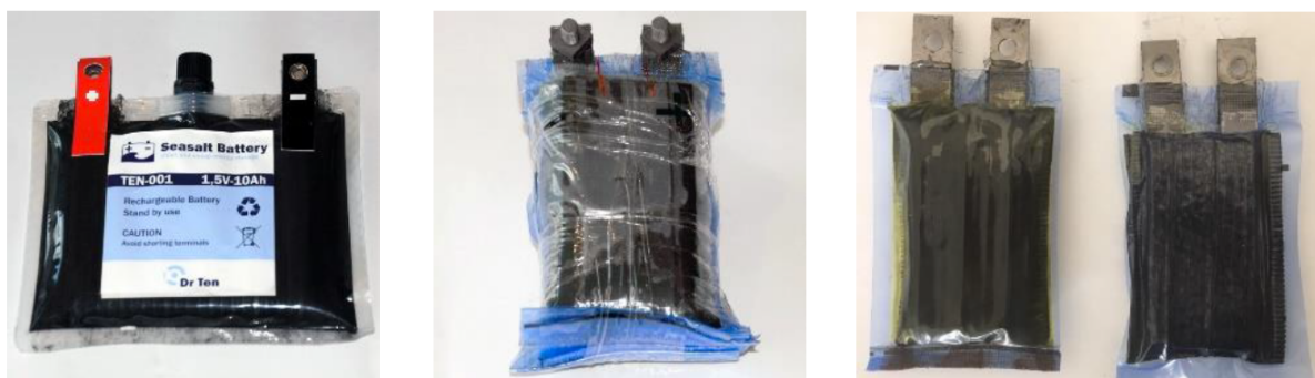
Figure 5. Illustration of the sea salt battery enclosures
