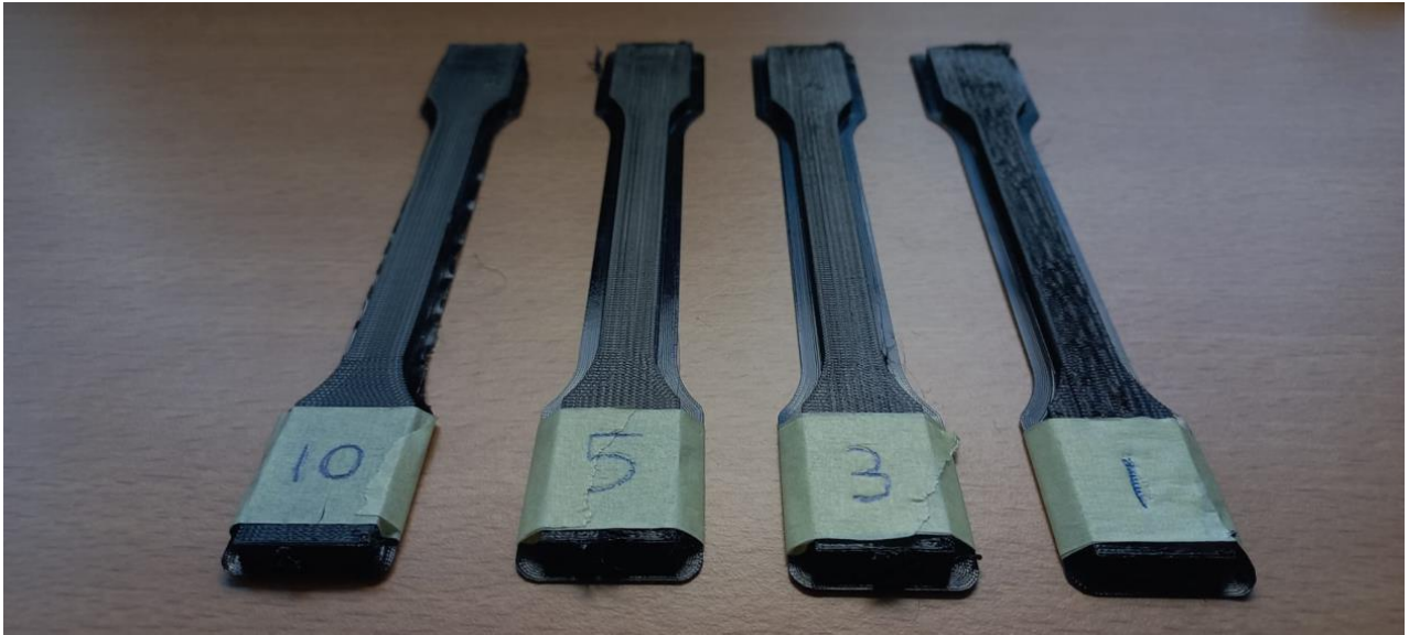
Varying iron speeds 10mm/s to 1mm/s
