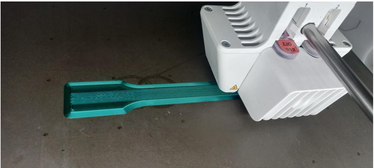
Figure X: Silk PLA dog bone being ironed with a offset of -0.05mm
