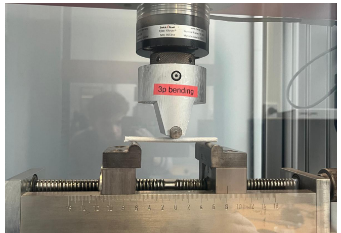
Figure 18: 3-point bending setup
