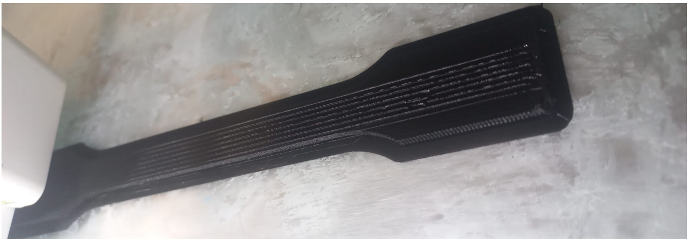
Figure 10: Regular PLA dog bone being ironed with a speed of 3mm/s
