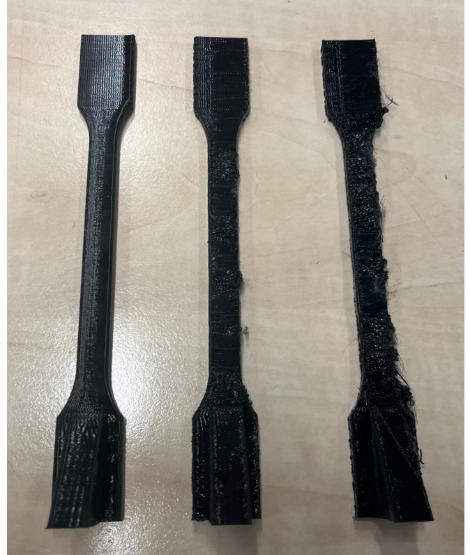
Figure 29: Ironing vertical specimen proved to be difficult. Unironed (left), Ironed (middle, right)
