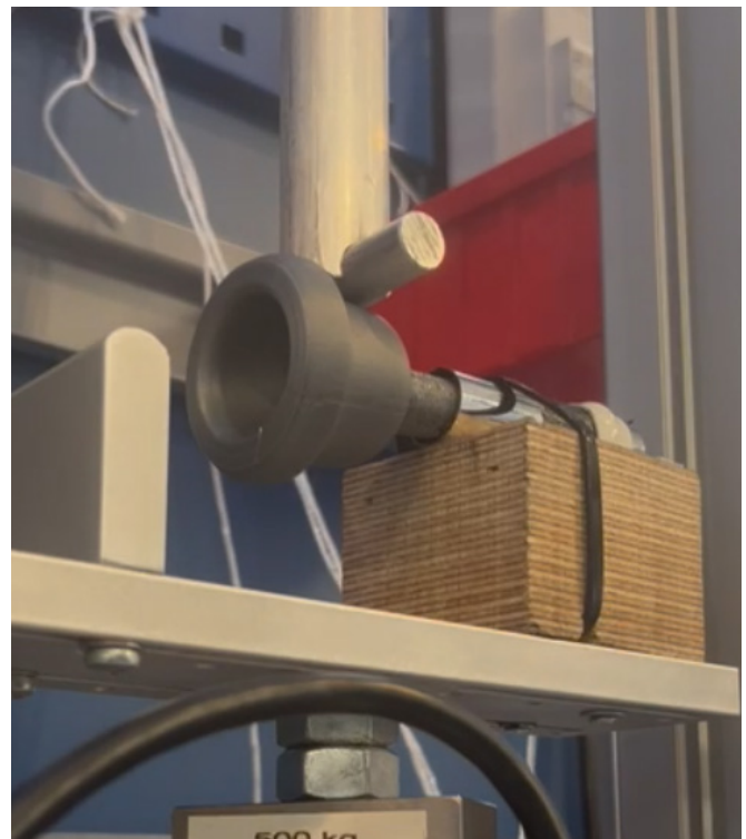
Figure 39: Flexural test trombone mouthpiece setup
