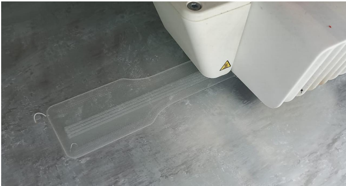
Figure X: Foaming PLA dog bone being ironed
