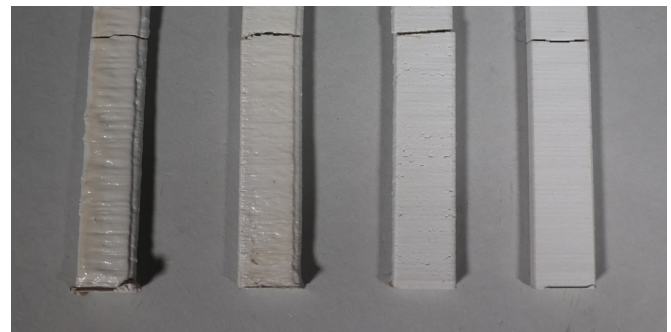
Figure 26: Effect of offset on outer surface of samples ironed with 3mm/s. (from left to right) No offset, 0.4mm offset, 0.8mm offset, Un-ironed
