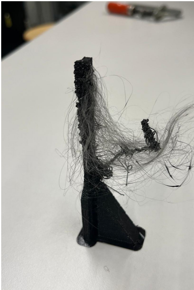
Figure 28: Severe stringing of vertical printed dogbone
