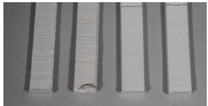
Figure 27: Effect of offset on outer surface of samples ironed with 5mm/s. (from left to right) No offset, 0.4mm offset, 0.8mm offset, Un-ironed
