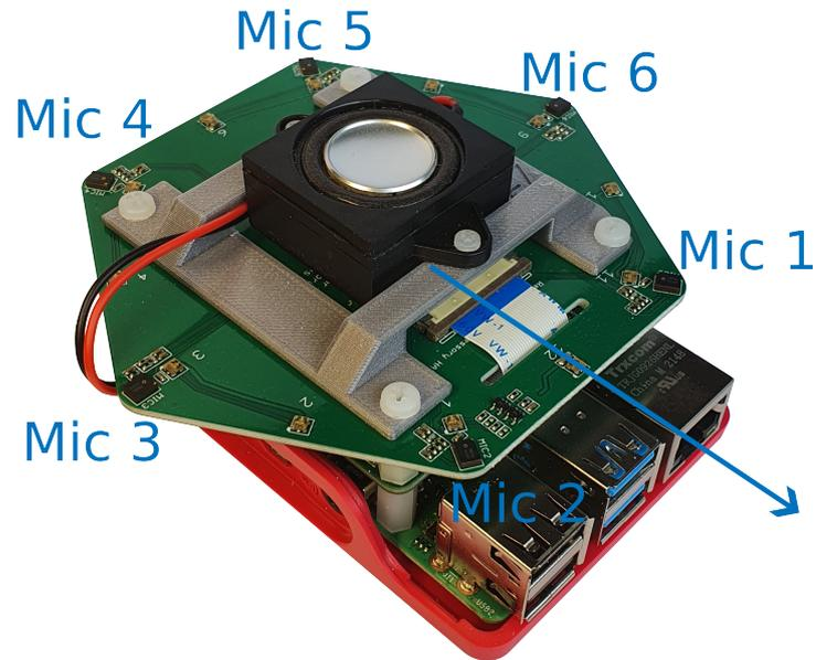
Figure 3.1: A Chirpy consisting of a Raspberry Pi 4 with the microphone array, accompanying shield and speaker stacked on top. Where the forward (or  $0^\circ$ ) direction is denoted by the blue arrow
