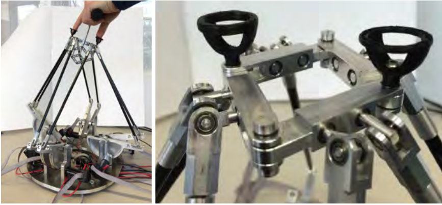
Figure 1.5: A parallel manipulator with two end-effectors enables gripping through the introduction of an internal closed-loop chain, here shown for a 7-DoF haptic device [23].
