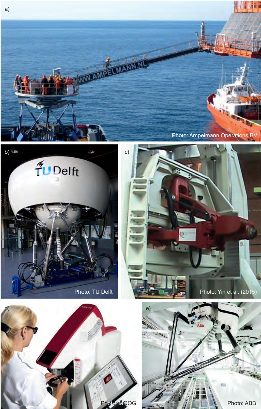
Figure 1.2: Parallel manipulators are applied in a wide range of applications, such as a) stabilization platforms [5], b) flight simulators [6], c) machining [7], d) haptic devices [8], and e) pick-and-place robots [9]
