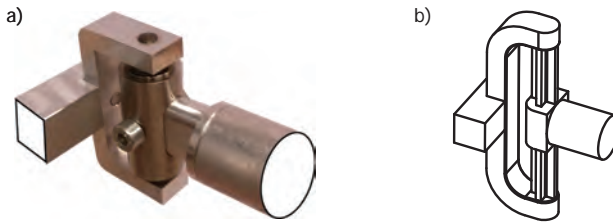
Figure 1.6: a) Traditional joints require significant design effort to prevent play, friction, and backlash, while they also suffer from wear. b) Compliant joints do not suffer from these effects and therefore pose an interesting alternative (image adapted from Trease et al. [30]).
