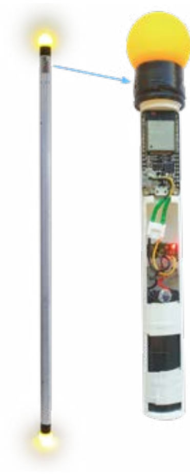
Figure 61: Testing prototype. left the overview right the probe that is inside with the battery, inertial measurement unit and arduino
