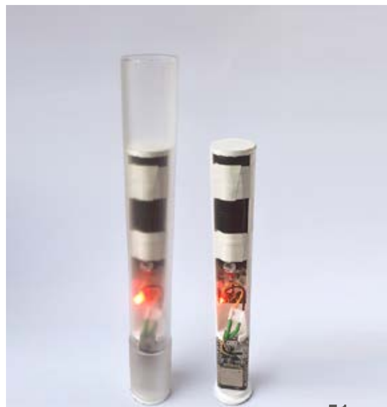
Figure 27: Arduino, IMU and battery inside a 3d printed housing
