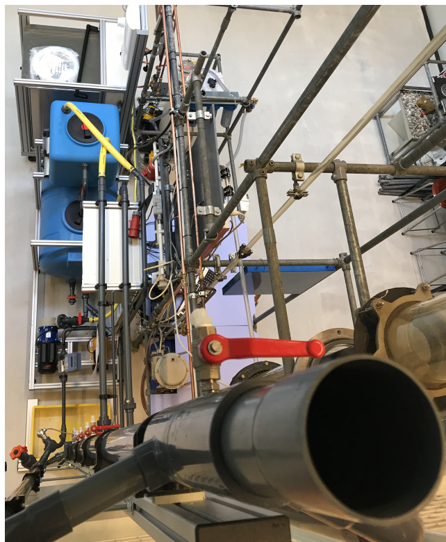
Figure 1. Experimental pilot set-up in Amsterdam, Utrecht, and London. D = 57 mm, with temperature control column (top view).
