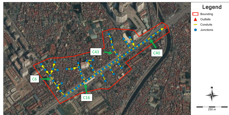
Figure C.2: 4 Conduits that were selected for simulating failure mechanism B: pipeline blockage.
