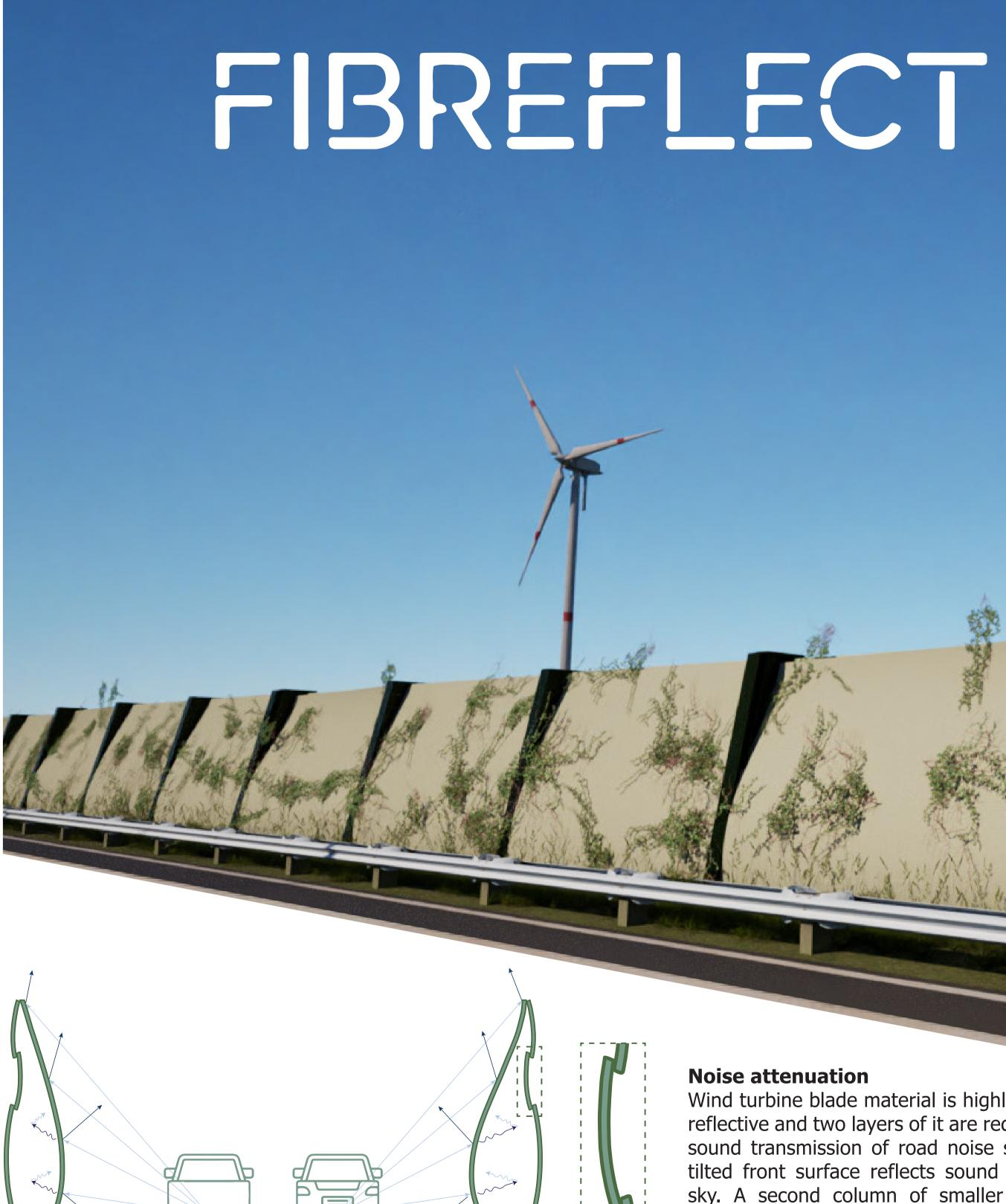
Ruben Gabriëls (R.J.) Design of a noise barrier from decommissioned wind turbine blades 26-02-2025 Integrated Product Design
