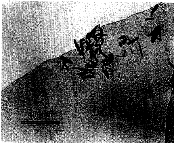
Figure 4.3. TEM photograph of the nano-apatite needles.
