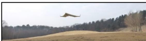
**Figure 2.1:** Flight test with glider model of the Flying-V, adopted from [13]
