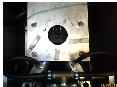
the caliper with compressed air cooling
