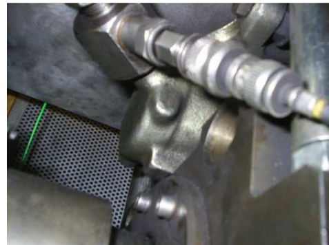
piezoelectric transducer of the hydraulic pressure
