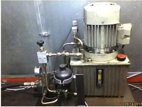
Figure 3.5 hydraulic pump with by-pass valve hydraulic line and the ABS servo-valve
