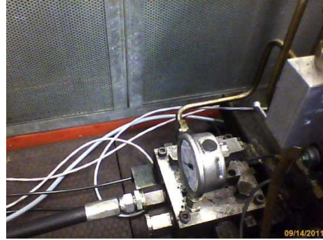
Figure 3.5 hydraulic pump with by-pass valve hydraulic line and the ABS servo-valve
