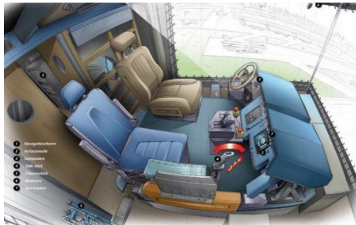
Figure 1: Illustration of HMI-Lab. The participant will be sitting on the right (blue) seat and controls the side-stick.
