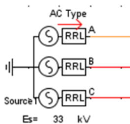
Figure 5. 33 [kV] voltage source.
