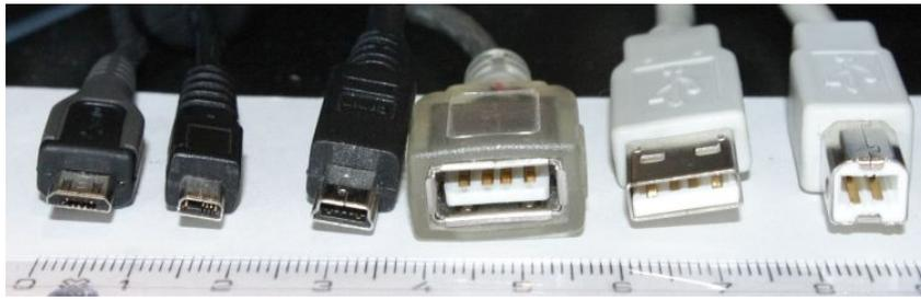
Figure 10.1: A variety of USB connectors. Note the clear presence of the four pins in all connectors: two differential signalling pins, one +5.0V pin and one ground pin. (Image courtesy: [61])
