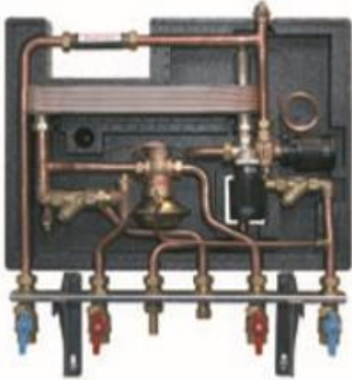
Figure 2-9 Supply set Orion from Danfoss. The supply set can receive DH water between 30 and 80 °C, and can control the return temperature to the district between 25 and 45 °C. Adapted from (Danfoss, n.d.)
