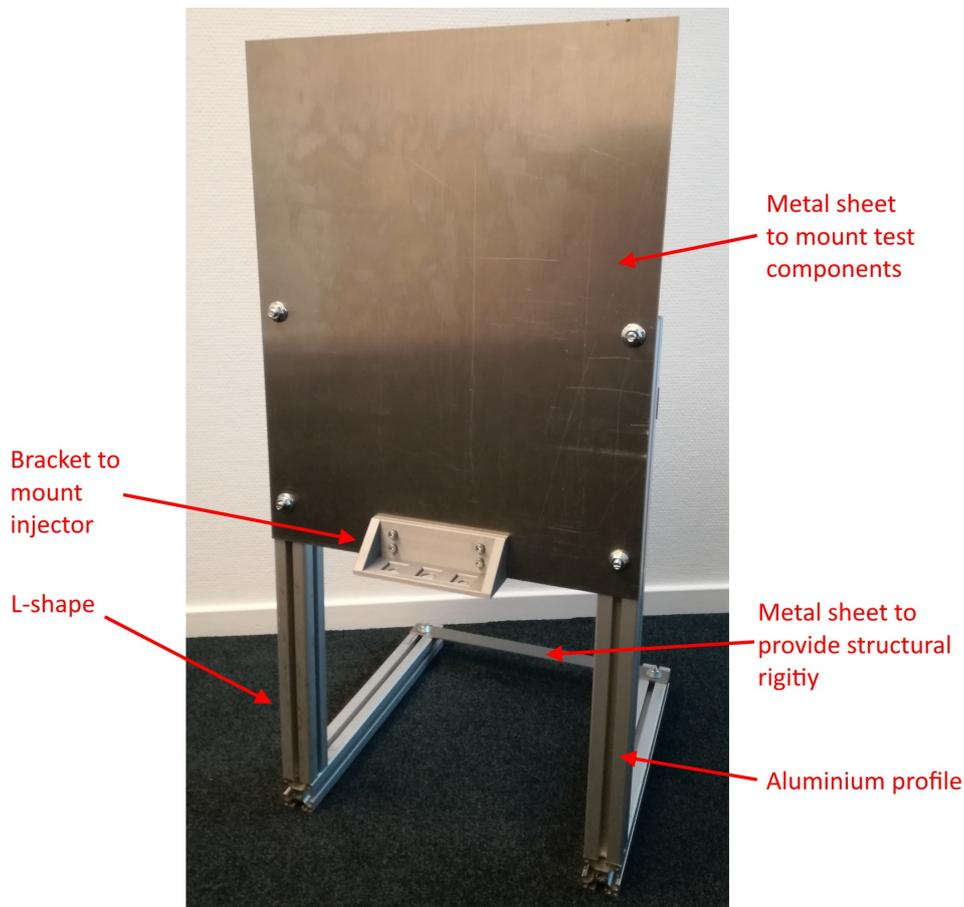
Figure 6.7: The constructed test stand, including bracket to mount the injector
