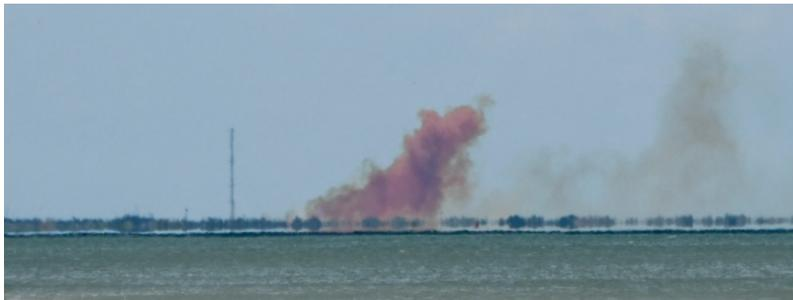
Figure 1.1: Example of a test anomaly during SpaceX crew Dragon where a toxic hydrazine cloud is formed [1]
