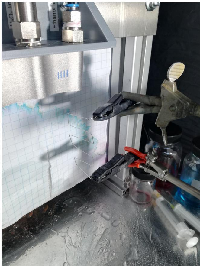
Figure 6.11: Clamping of the heating element
