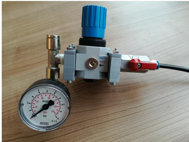
Figure 6.5: Section of the test setup for the compressed air feed line
