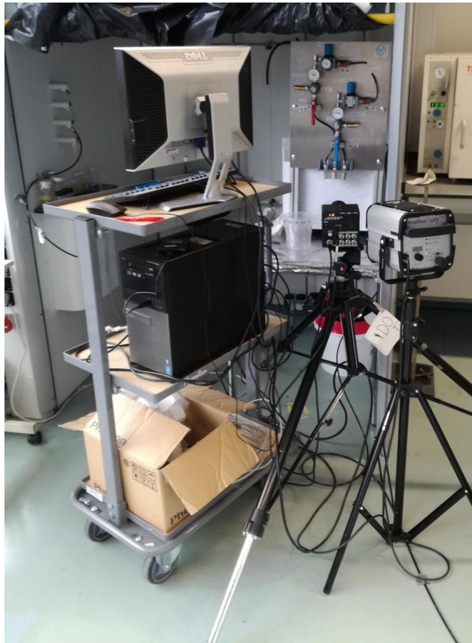
Figure 6.10: Overview of the placement of the test setup, high speed camera and external light source
