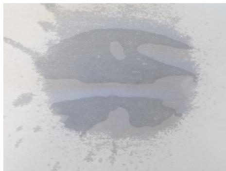
Figure 7.16: Spray pattern of the two jet injectors of configuration 4
