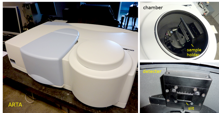
Figure 2.7: The photograph of Automated Reflectance Transmittance Analyzer (ARTA) installed in the PerkinElmer ® Lambda ™ 950 Spectrophotometer.
