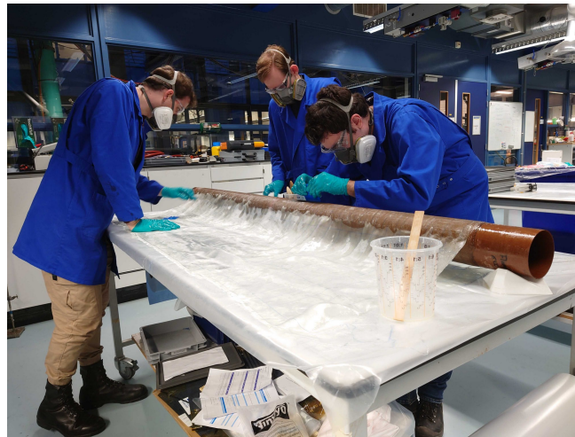
Figure 3.2: Manufacturing of the “Puffin” rocket motor using a wet-layup technique (author on left)
