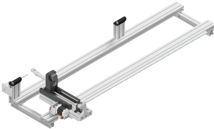
Figure 4.2: Render of the filament winder used for manufacture of the test samples. Filament is supplied pre-tensioned from the lower left corner of the figure, passing around the redirection rollers and through the delivery arm to the delivery roller, which stands around 2 cm from the mandrel surface. The mandrel is suspended along the axis provided along the upper left extrusion.
