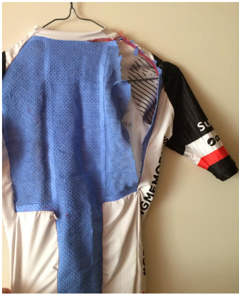
Figure 39. Failure of design due to stretching
