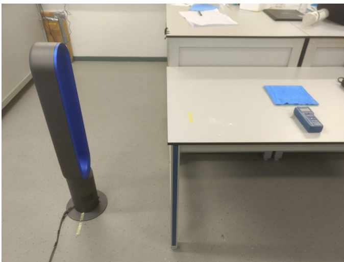
Configuration used in the experiment to get 1.5m/sec wind speed over the PVA sample
