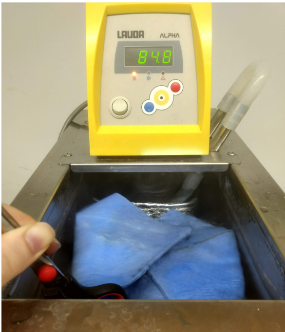
Figure 21. Heating the PVA towel with hot water
