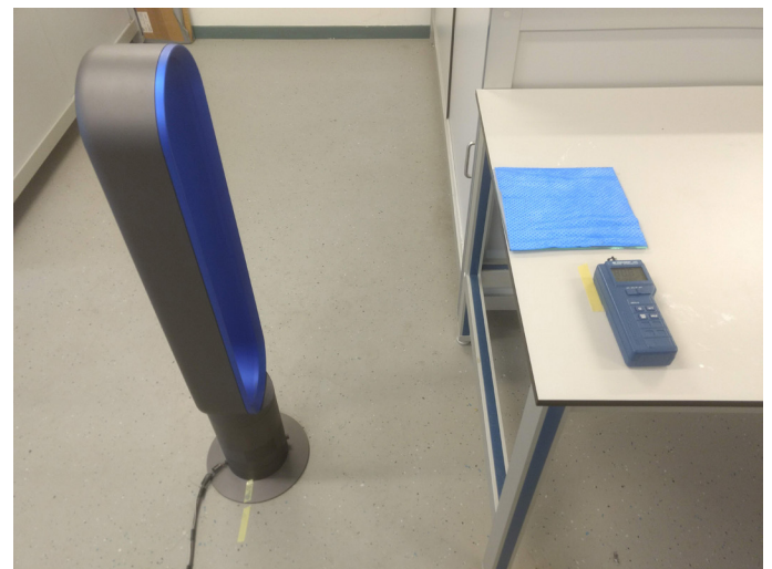
Configuration used in the experiment to get 2.5m/sec wind speed over the PVA sample
