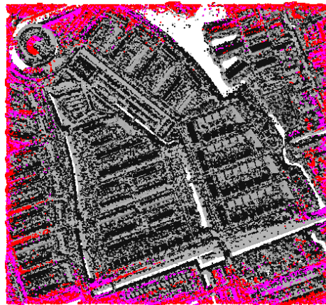
Figure 3.4: Points with a successfully created medial axis are displayed in grayscale. Points which are not finished processing because they need to know the location of points outside the region are displayed in red or purple. They represent the inner and outer MAT respectively
