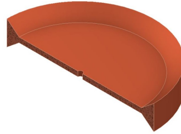
Figure D.11: Cross section ISO view of flywheel with linear increasing thickness.
