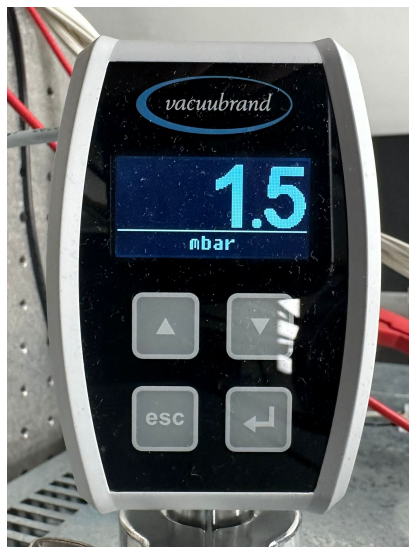
Figure 6.20: The digital barometer attached to the vacuum chamber, measuring 1.5 mbar .
