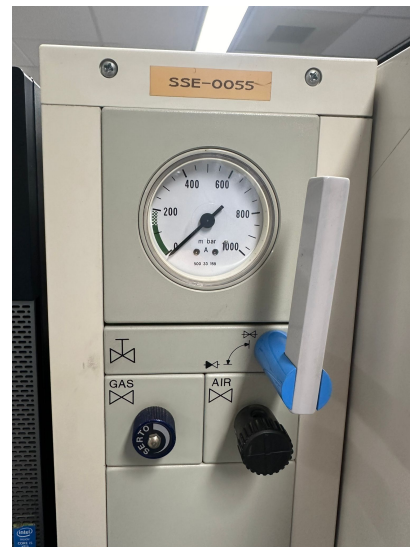
Figure 6.21: The analogue barometer embedded into the vacuum chamber, measuring 1.5 mbar .
