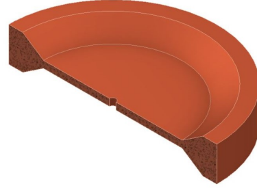
Figure D.17: Cross section ISO view of flywheel with hybrid linear design.
