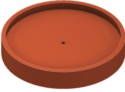
Figure D.4: ISO view of flywheel with stepped uniform thickness.
