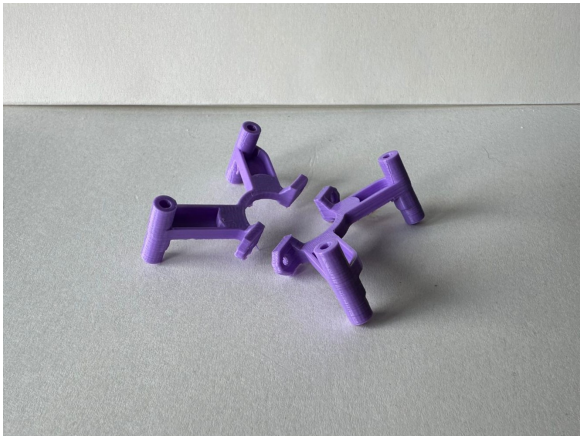
Figure 5.6: The prototype body printed using a FDM printer, treated using hand tools to ensure acceptable margins.
