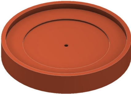
Figure D.7: ISO view of flywheel with hybrid stepped design.
