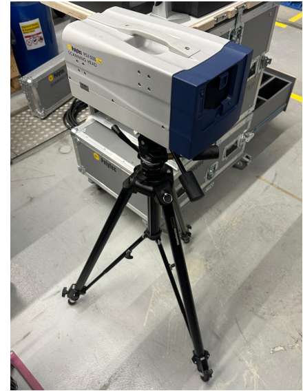
Figure 6.15: The PSV-500 Laser Vibrometer scanning head.
