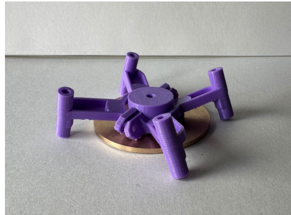
Figure 5.7: The prototype body enclosing a dummy print of the Faulhaber motor and the flywheel for scale.
