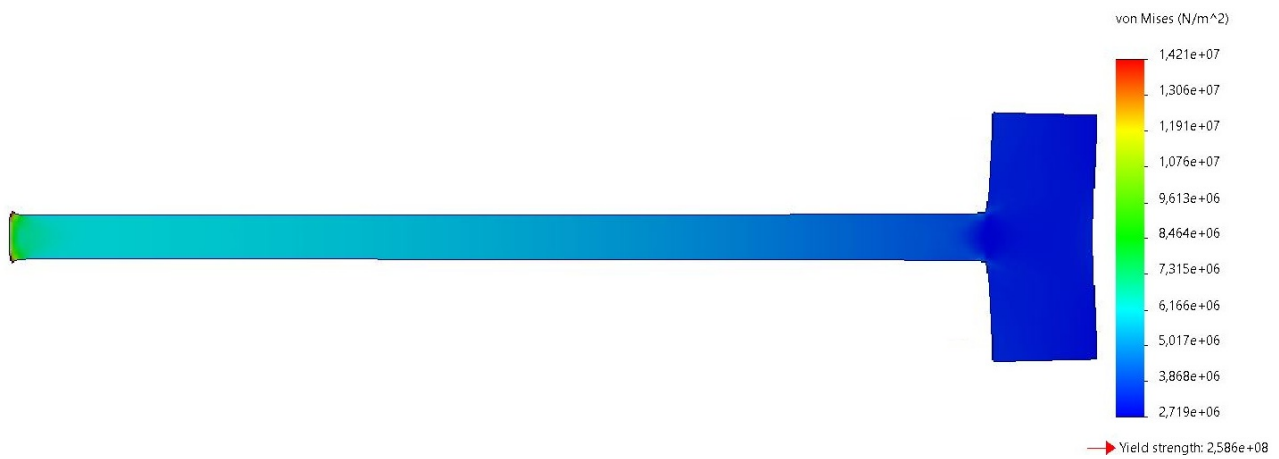
Figure 4.9: The deformed stress simulation result for a symmetrical stepped design at a deformation scale of 6000.
