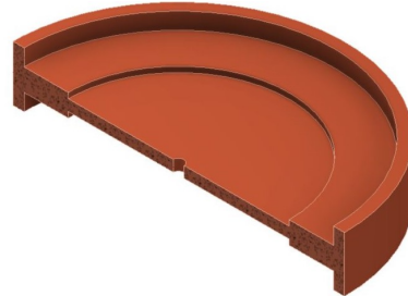
Figure D.8: Cross section ISO view of flywheel with hybrid stepped design.
