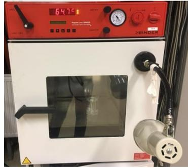
*Figure 53 The oven for heating up the water-oil emulsion cans*
