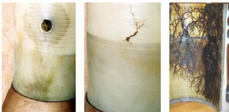
*Figure 5 Electrical faults in the oil termination due to water contamination [4].*
