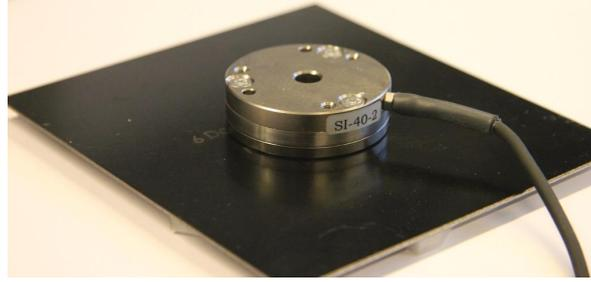
**Figure 3.7:** The actuator forces and torques were measured with a 6-DoF force sensor. One side of this sensor was mounted to the moving stage and the other side to the measurement frame by means of a temporary support structure.
