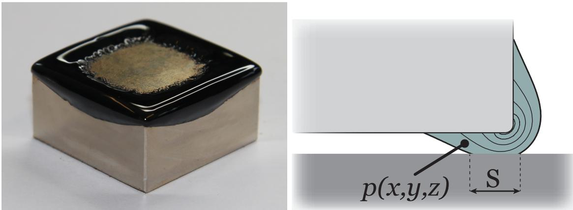
**(a)** Ferrofluid moves to the region of the highest gradient field, which is on the edges of a (square) permanent magnet.
