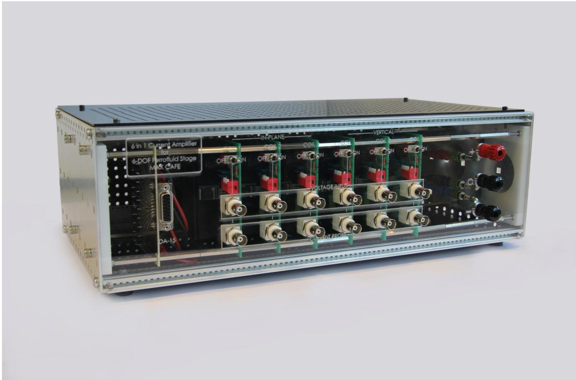
**Figure 6.5:** The six current amplifiers are assembled into one amplifier box. All output signals are transferred to the PCB via a D-Sub 15 cable.
