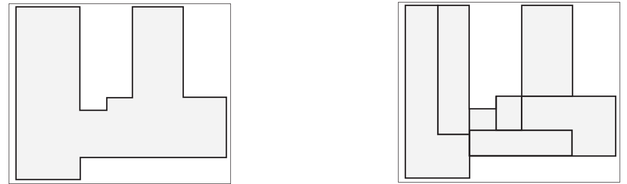
Figure 43. Thermal zone division, (Left) Single zone, (Right) Detailed zone, Energy Plus manual (2015)
