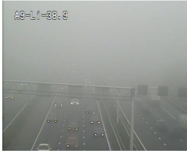
Figure 6.9: Image with a visibility of more than 250 meters. The camera is zoomed in, making it appear more foggy than it actually is. The matrix boards on the right are 250 meters away from the camera and are clearly visible. Therefore, the visibility is above 250 meters, and the image should be labeled as "clear".
