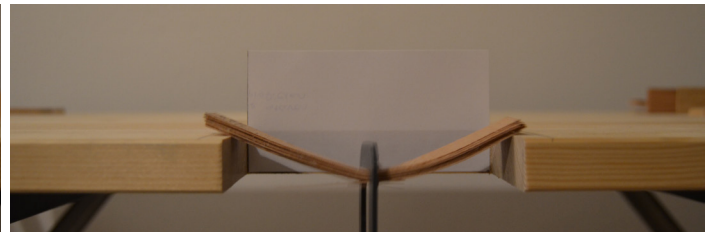
Figure 28 - Multiple direction beech veneer 0.5mm 8ply Max load of 108.85 N
