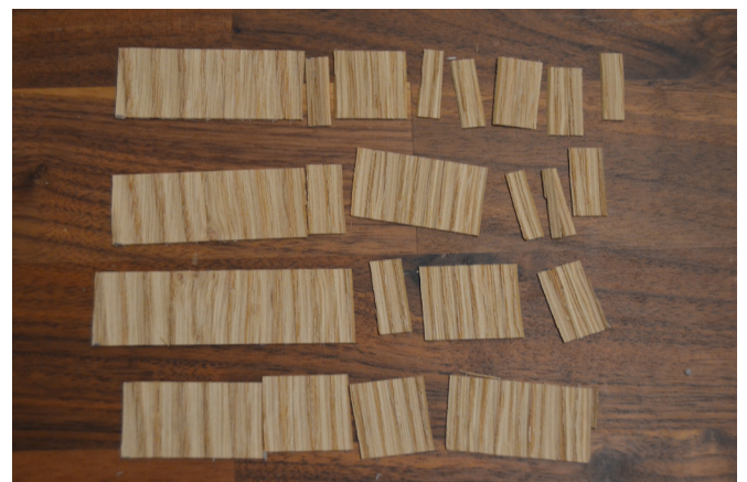
Figure 23 - Oak veneer falling apart after cutting (author)
