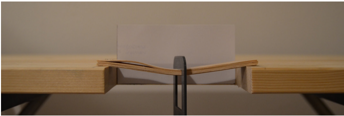
Figure 25 - Linear birch veneer 0.6mm 8ply - Max load of 103.95 N
