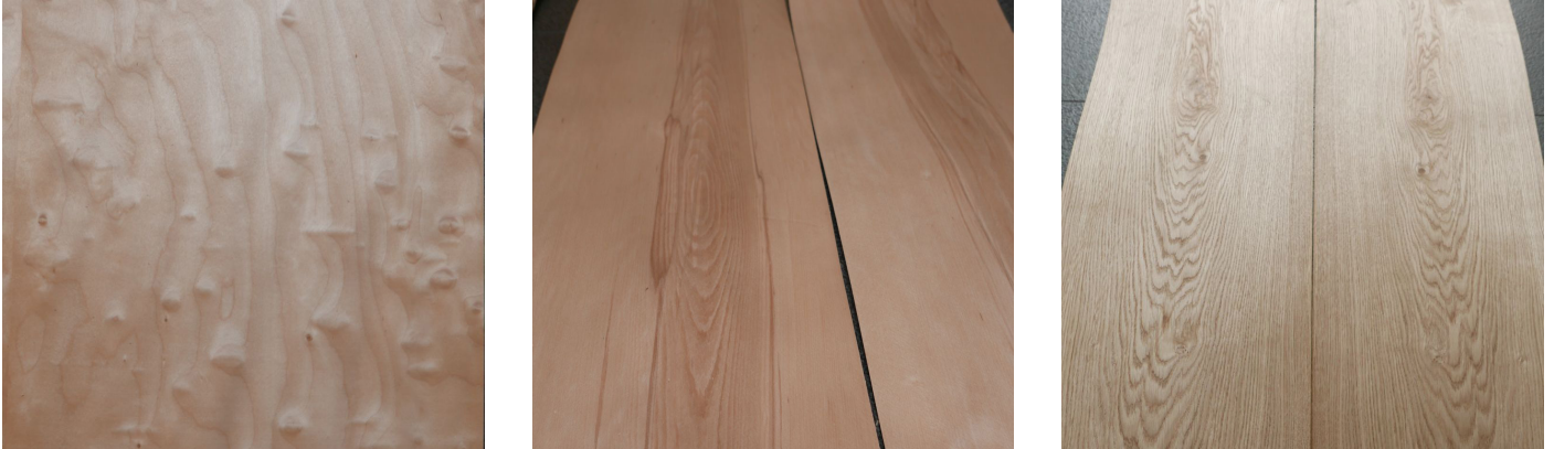
Figure 20 - Birch, beech and oak veneer used as base material for the sample (author)
