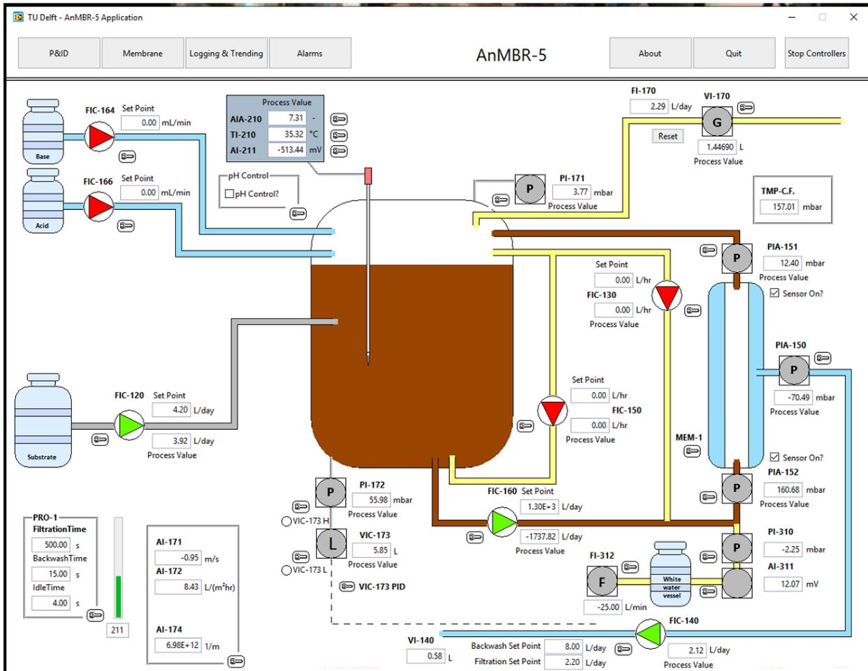
Figure 18 Computer interface of the reactor
