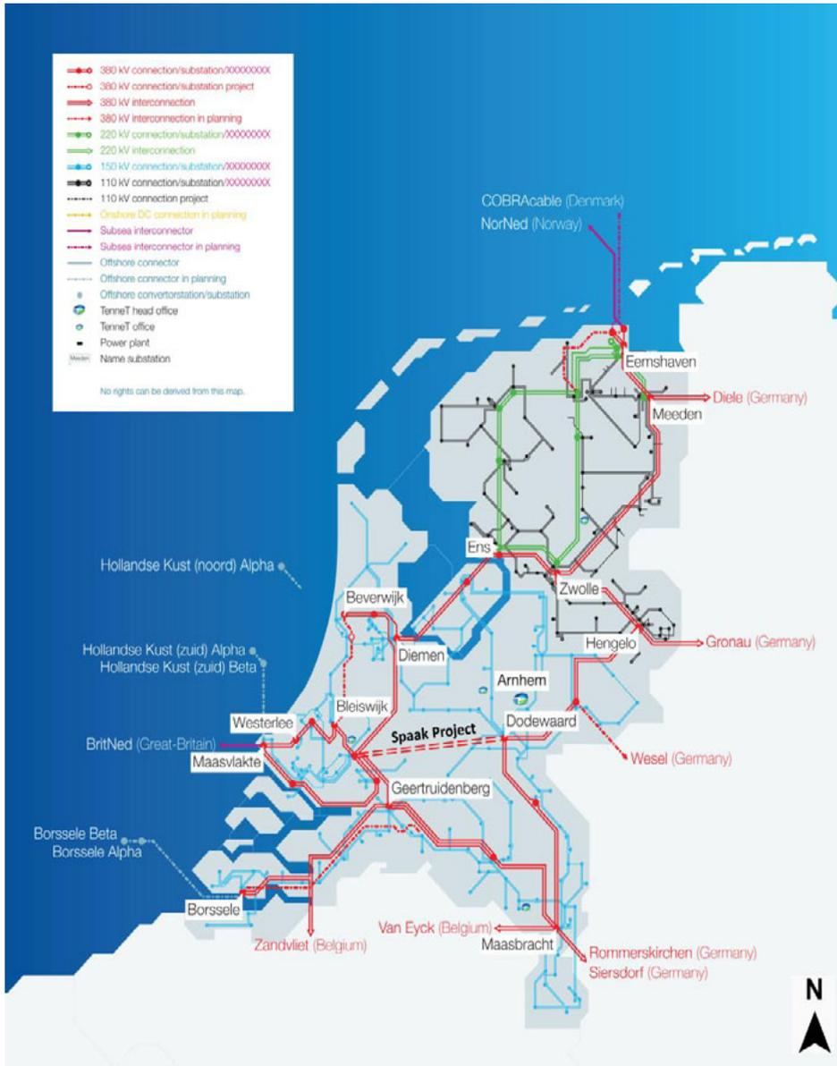
Figure 2.1: Map of the Dutch (E)HV transmission grid. [Source: TenneT TSO, 2018]
