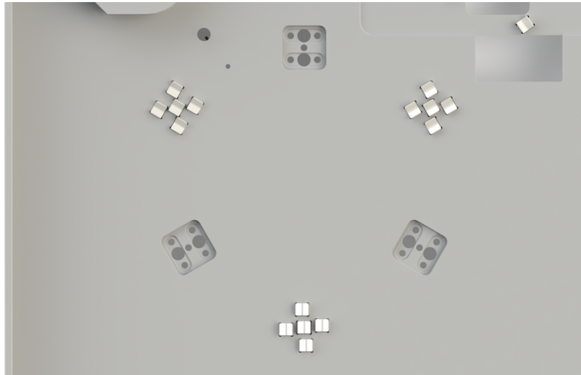
Figure 4.22: The 3 integrated v-groove islands and the 3 locations of the flexure connection.
