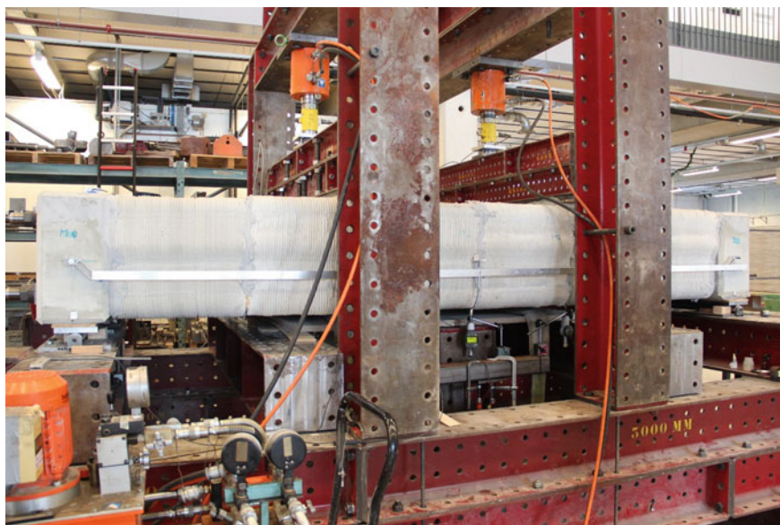
Fig. 2.6 Scale model in 4-point bending test set-up
