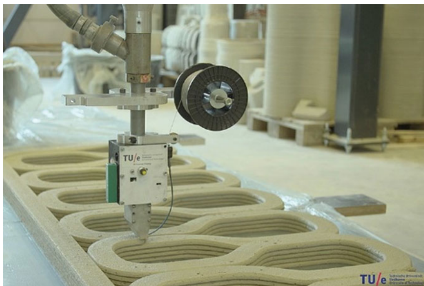
Fig. 2.3 Printing of a bicycle bridge element
