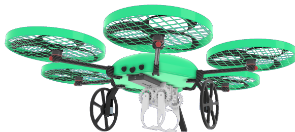
Figure 2: Visual representation of the drone with the grabber pick-up mechanism
