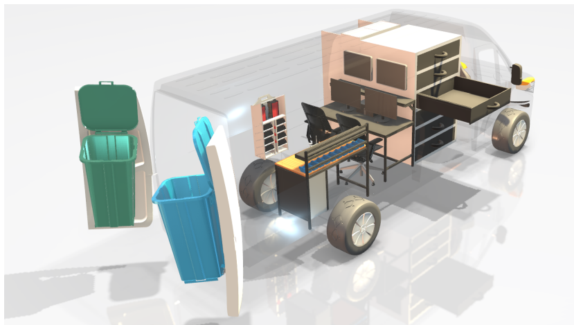
Figure 4: Render of the ground station with transparent van body
