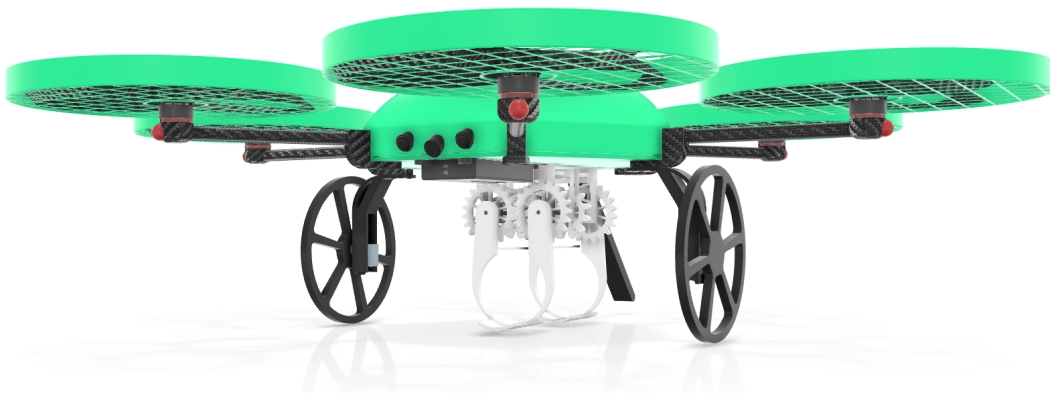
Figure 5.27: Render of the drone with the grabbing mechanism made in 3DEXperience
