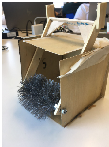
Figure 5.4: Prototype model of the brush mechanism
