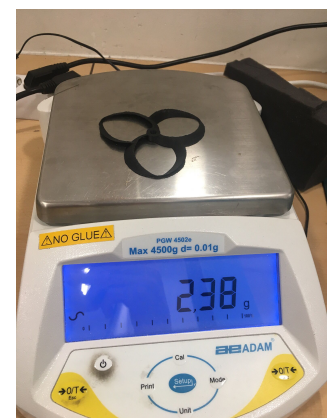
(c) Toroidal propeller used in testing with its mass
