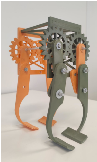
(a) 3D printed prototype of the pick-up system, the green grabbing mechanism represents the first iteration, while the orange one represents the final iteration
