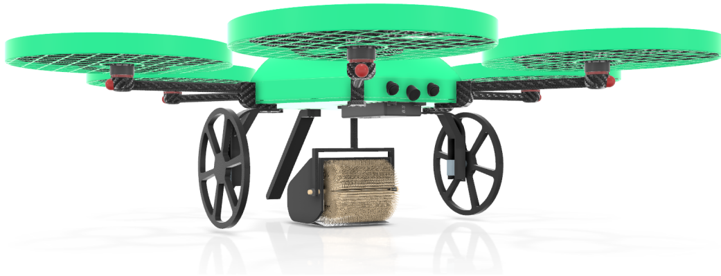
Figure 5.28: Render of the drone with the brushes mechanism made in 3DExperience
