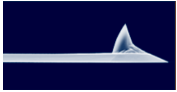
(b) Tip set back with approximately 15 \mu\text{m} . Image source: www.budgetsensors.com
