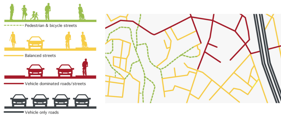
Fig. 1.13 Four different street profiles including functions as classified by van Eldijk (left) and translations of these into a map of the Grefsen area in Oslo (right)
