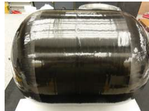
Figure 7.22: Carbon wound pressurant tank for He
