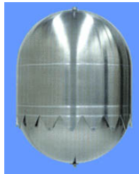
Figure 7.21: Tension surface tank for MMH and MON
