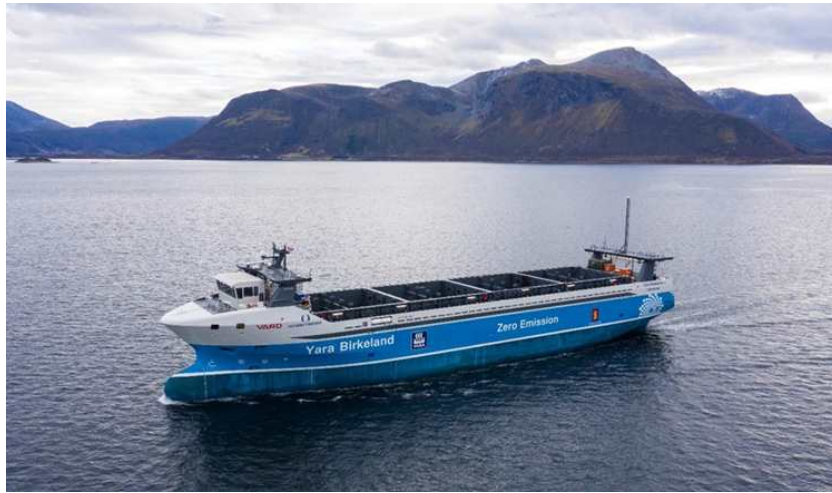
Figure 1.3: The YARA Birkeland, the world's first fully electric and autonomous container ship with zero emissions. [5]
