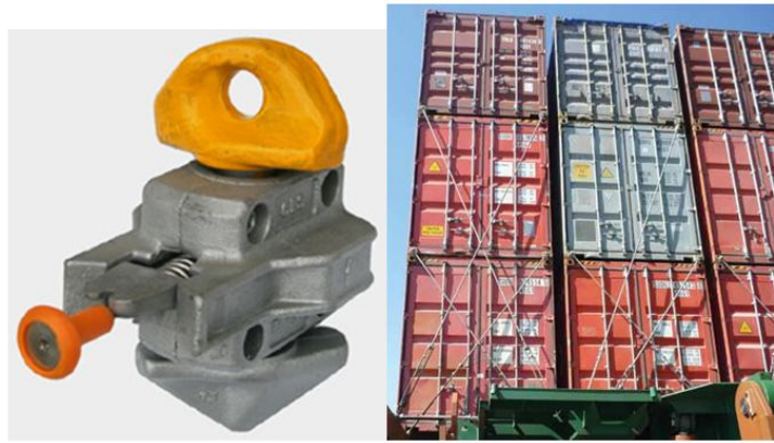
Figure 9-5 Left: Semi-automatic twistlock [64], Right: Containers supported by lashing rods [65]
