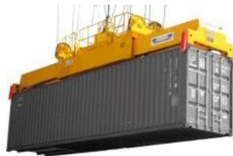
Figure 9-11 Container being lifted by a spreader [71]
