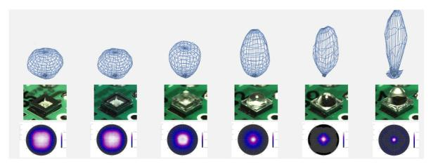
Figure 5.1: Measured Radiation Characterization
