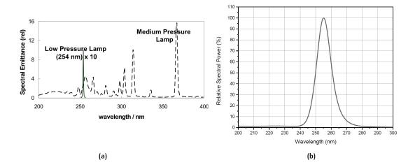
Figure 1.3: Power Distribution of (a) Tradition Mercury-vapor lamp spectrum (b) UV- LED spectrum
