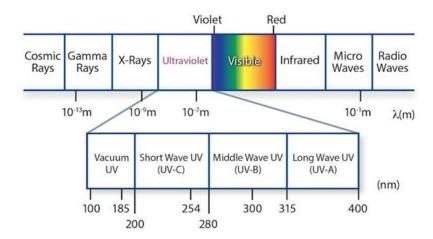
Figure 1.1: Ultraviolet in Electromagnetic spectrum
