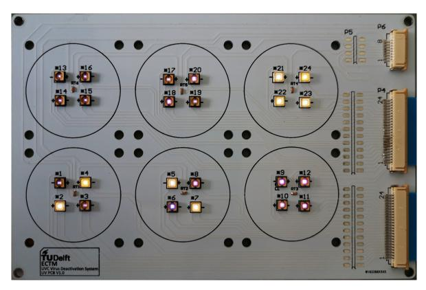
Figure A.1: LEDs illumination status of UV-C LED Array
