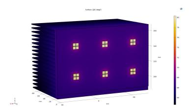
Figure 2.6: Thermal Simulation of UV-C LED Array with Cooling module
