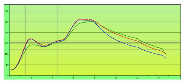
Figure A.5: Soldering profile for UV-C LED Array
