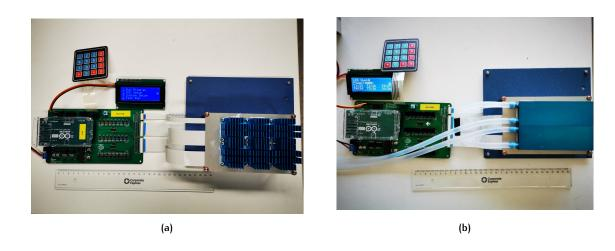
Figure 2.14: UV-C LED Platform (a) Air Cooling version (b) Liquid Cooling version
