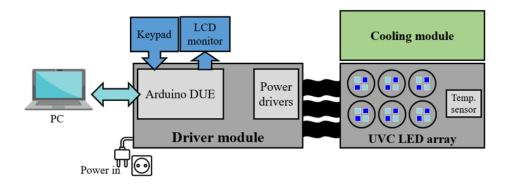
Figure 2.3: System Diagram of UV-C LED Virus Inactivation Experimental Platform
