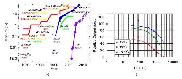
**Figure 1.4:** (a) DUV LEDs performance (b) Decay of output power of 280 nm LEDs during aging tests for varying junction temperatures
