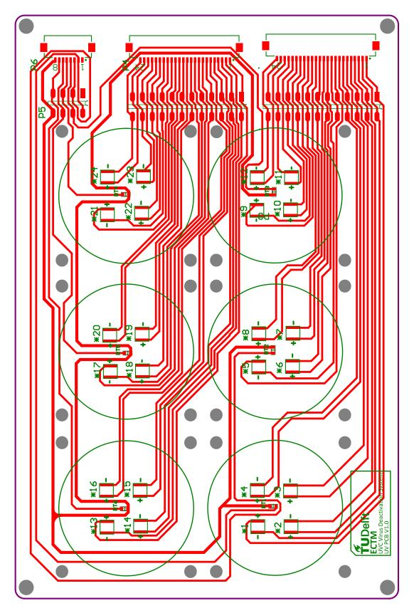
Figure B.1: PCB design file of  $\mathit{UVC\ Virus\ Inactivation\ Test\ Platform}$
