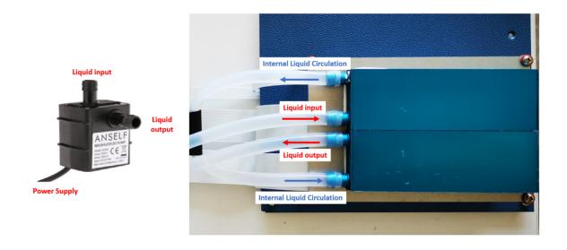
Figure 2.8: Water Circulation of Cooling module
