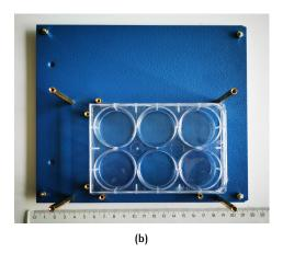
Figure 2.7: Structure of (a) UV-C LED array and Cooling module (b) Alternative Cell Culture Plate
