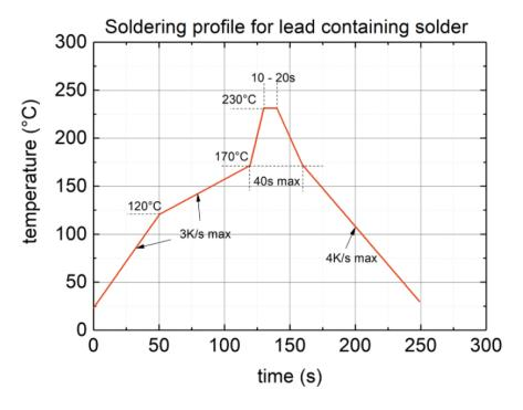
Figure A.3: Soldering profile for lead containing solder
