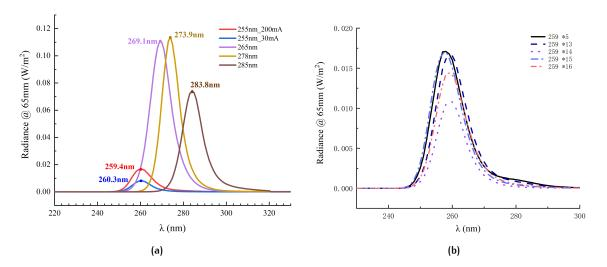
Figure 2.17: Characterization of (a) Overall Radiance Power and Peak wavelength measured at maximum power step (b) Radiance Power variance and Peak wavelength shift of nominal 255 nm LED
