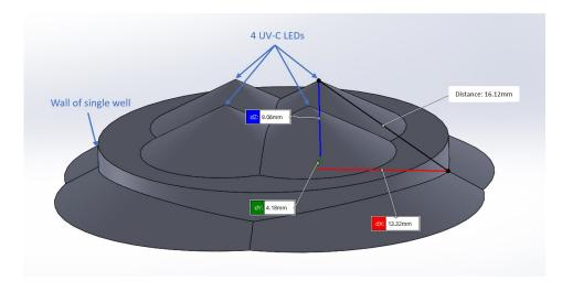
Figure 2.19: 3D illumination model of single well
