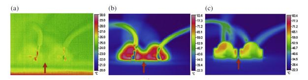
Figure 2.5: Effect of the PCB material on the heat dissipation of LEDs at 0.3 A. (a) LEDs held in series on a PCB at room temperature without current supply initially, (b) LEDs on a FR4 PCB, and (c) LEDs on a metal core PCB
