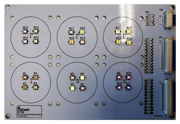
Figure A.2: LEDs illumination status of UV-C LED Array
