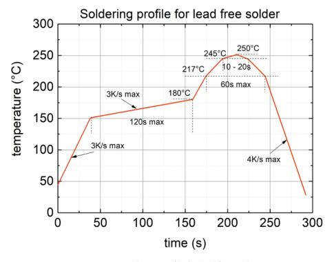
Figure A.4: Soldering profile for lead free solder
