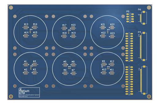
Figure 2.9: UV-C LED Array
