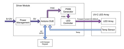
Figure 2.10: Driver Module Composition
