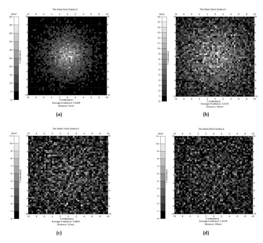
Figure 2.4: Irradiance Simulation of single ultraviolet LED a) 5 mm, b) 10 mm, c) 17 mm, d) 20 mm exposure distance
