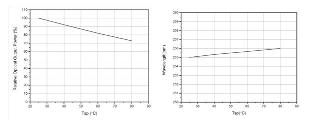
Figure 2.2: Relative Optical Output Power vs. Solder Point Temperature, IF=100 mA (left), and Peak Wavelength vs. Solder Point Temperature, IF=100 mA (right)
