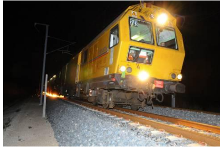
Figure 28: Maintenance grinding train
