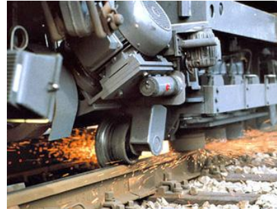
Figure 29: Detail of grinding process
