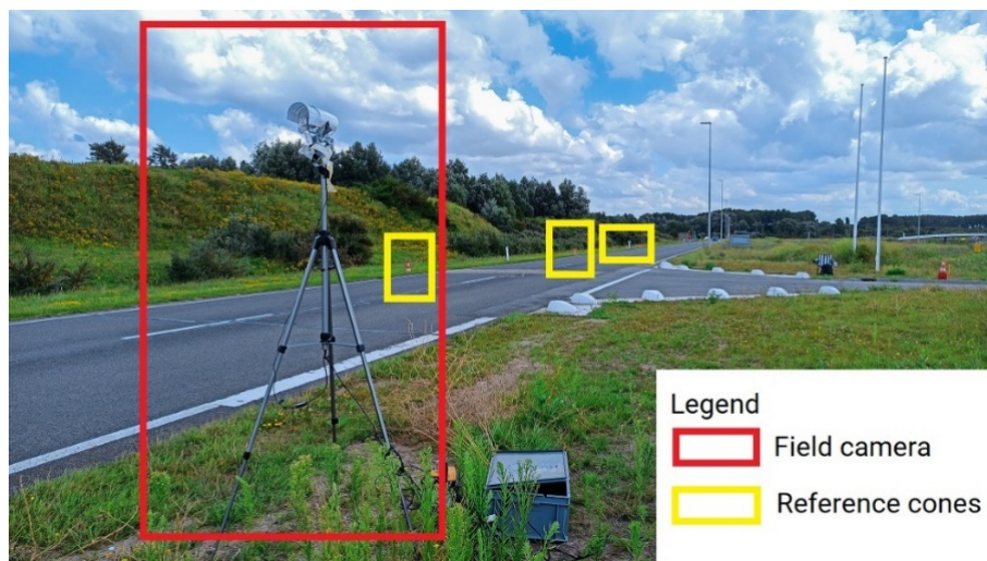
Figure 2.6: Field camera and reference cone setup near the parking lot - point B.
