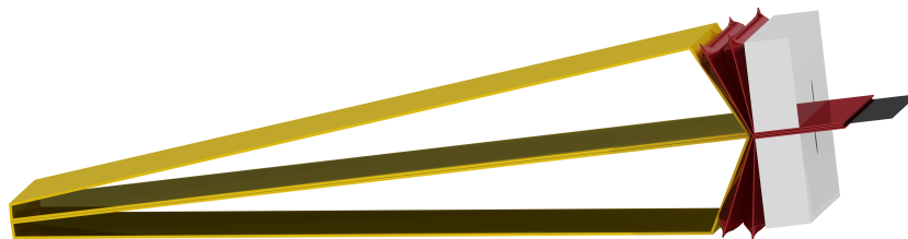
Figure 5.1: Rendering of the test object with the bellows in red, spars in grey, trailing edge in yellow and inner sheet in black
