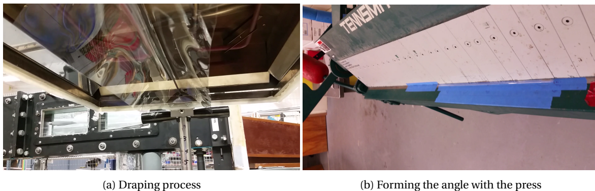
Figure 4.1: Production processes of the bellows
