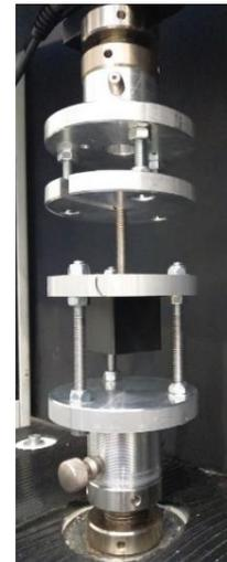
**Figure 3-2:** Test-setup for the pull-out tests
