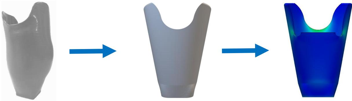
**Figure 2-4** Initial socket design was measured and those dimensions were converted into simplified STL model. With the values of forces and contact pressure found in literature bounding conditions were set and an FEA of the socket was executed.
