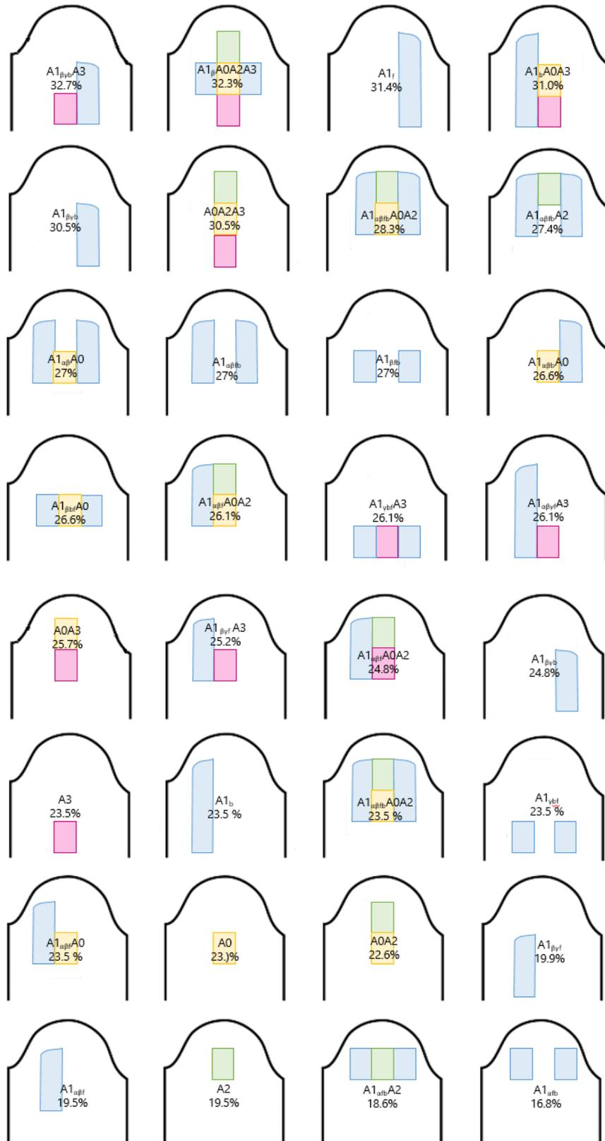
**Figure B-2:** Results of 47 FEA reinforcement combinations to determine the area of effectiveness. Expressed in stress reduction in %.
