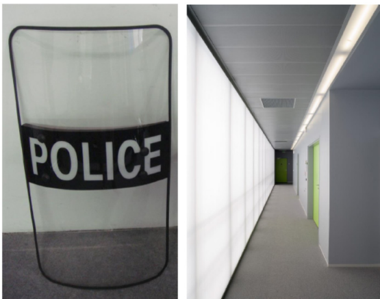
Figure 6.3.1.4: Polycarbonate shield and Light transmission through polycarbonate facade panels ( http://www.iplasticsupply.com/ ) ( http://www.archdaily.com/9218/hq-13-parisian-subway-line-atelier-phileas/ ).
