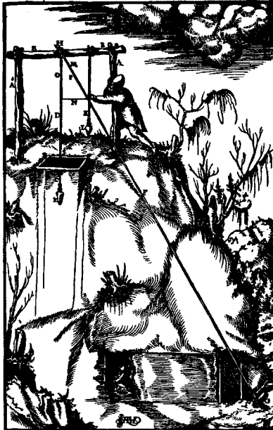
A—UPRIGHT FORKED POSTS. B—POLE OVER THE POSTS. C—SHAFTS. D—FIRST CORD. E—WEIGHT OF FIRST CORD. F—SECOND CORD. G—SAME FIXED GROUND. H—HEAD OF FIRST CORD. I—MOUTH OF FUNNEL. K—THIRD CORD. L—WEIGHT OF THIRD CORD. M—FIRST SIDE MINOR TRIANGLE. N—SECOND SIDE MINOR TRIANGLE. O—THIRD SIDE MINOR TRIANGLE. P—THE MINOR TRIANGLE.
