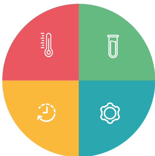
Figure 20: The Sinner circle, which contains the four elements that influence the effectiveness of cleaning: the mechanical action of the cleaning fluid, the cleaning time, the temperature and the chemical reaction.
