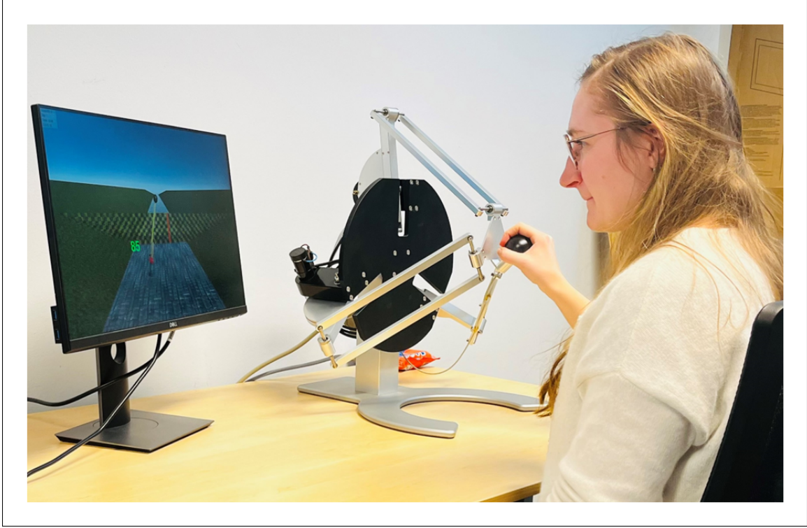
Fig. 1: Experimental Setup with a participant interacting with the Force Dimension Delta.3 robot when playing the pendulum Game.
